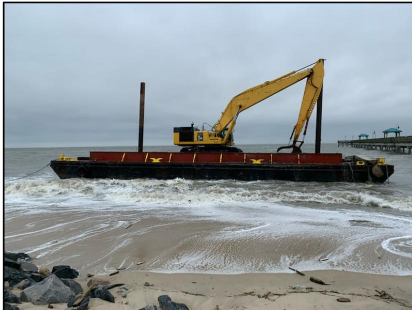
The *YD71* aground after breaking free from its mooring and prior to striking the pier. (Source: U.S. Coast Guard)
