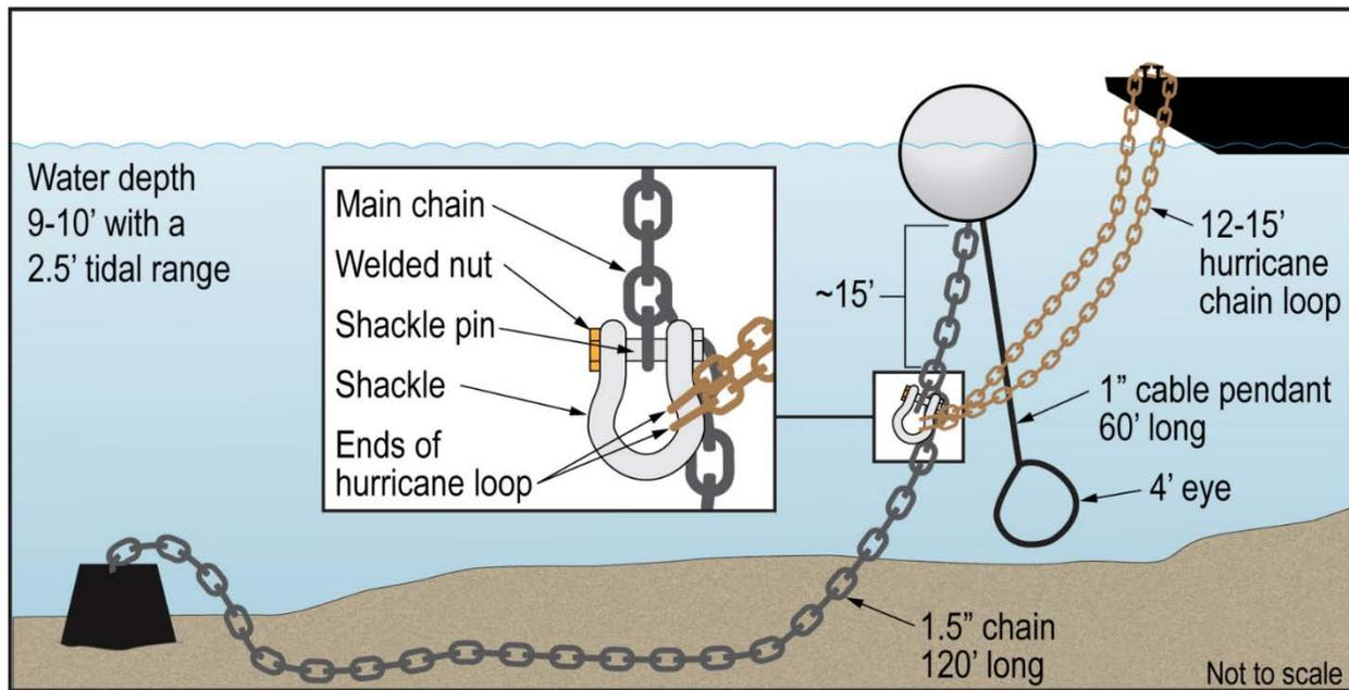
A representation of the arrangement of the YD 71's mooring at the time of the accident.
