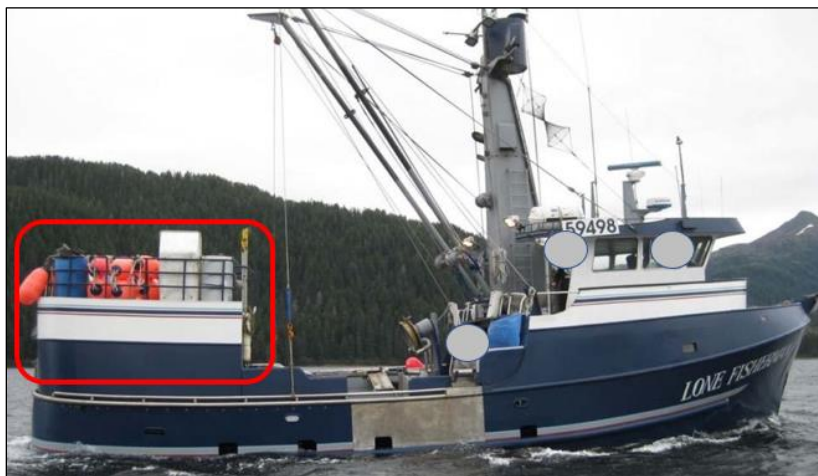
Left; undated photo of the Pacific Knight (then named the Lone Fisherman ) with the aft deckhouse that was removed (highlighted in red). Right: the Pacific Knight while moored alongside a dock on June 10, 2018, with the two added cranes. (Photos courtesy of Lone Fisherman, LLC)
