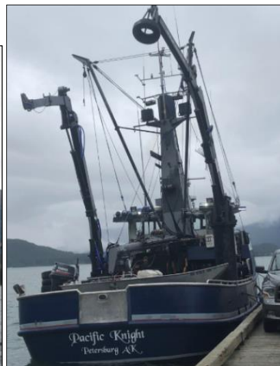
Left; undated photo of the Pacific Knight (then named the Lone Fisherman ) with the aft deckhouse that was removed (highlighted in red). Right: the Pacific Knight while moored alongside a dock on June 10, 2018, with the two added cranes. (Photos courtesy of Lone Fisherman, LLC)
