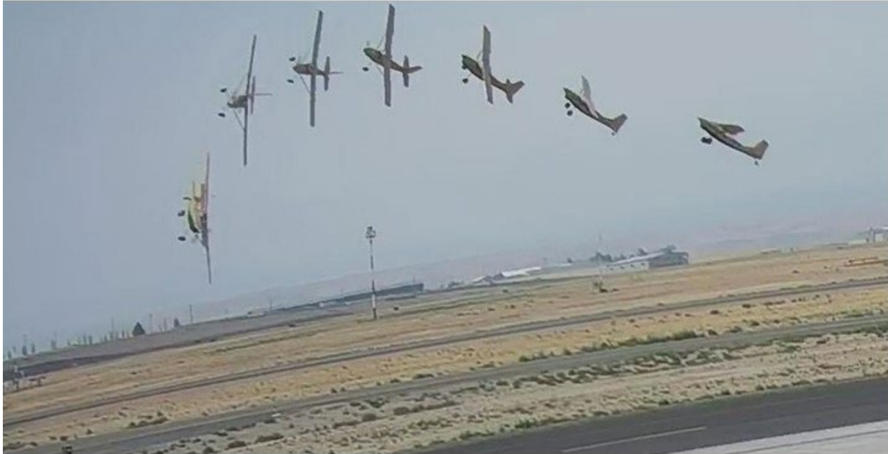
Figure 1. Composite Image Showing the Airplane between 3.7 seconds and 7.3 seconds after Takeoff
