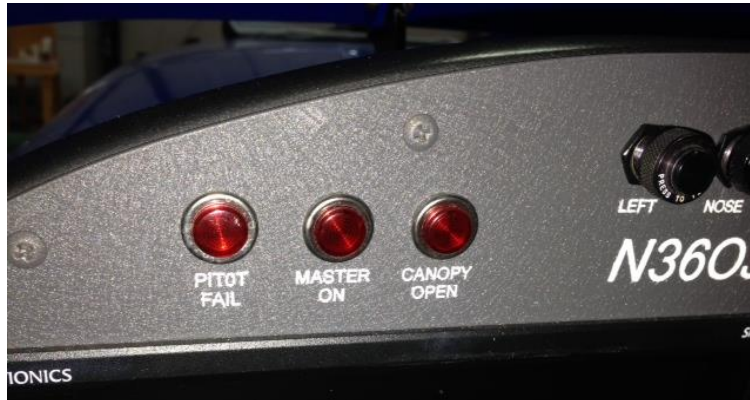
Example Canopy Unsafe Warning Light in Jack Addison's Lancair 360
