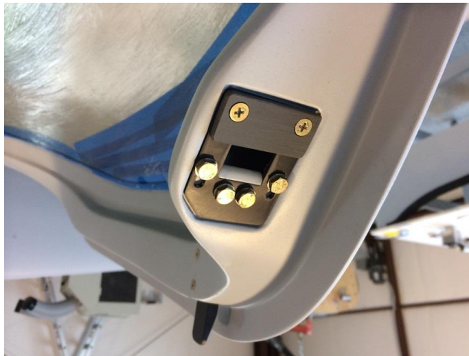
Photo of Canopy Striker Modified with Lift Plate Installed
