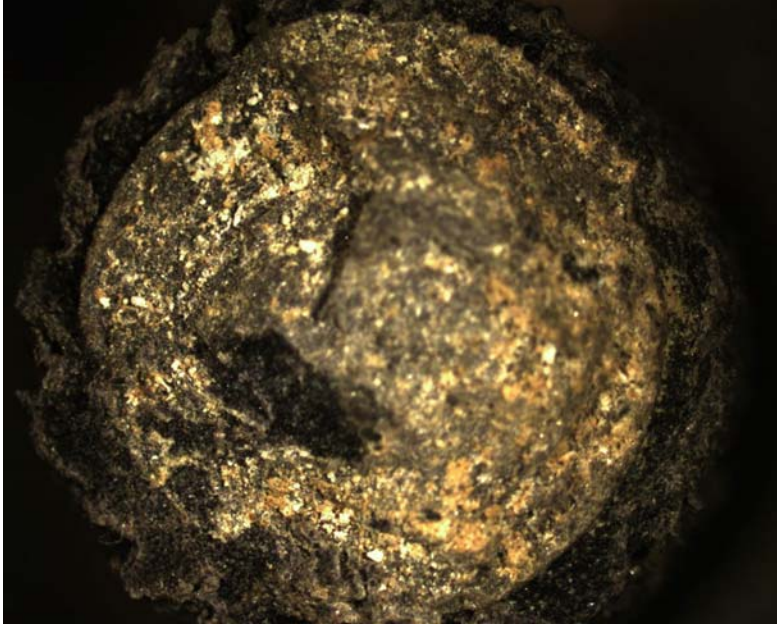
Figure F1: Sample 07-1090 Back Left (threaded end) Fracture Surface As-Received
