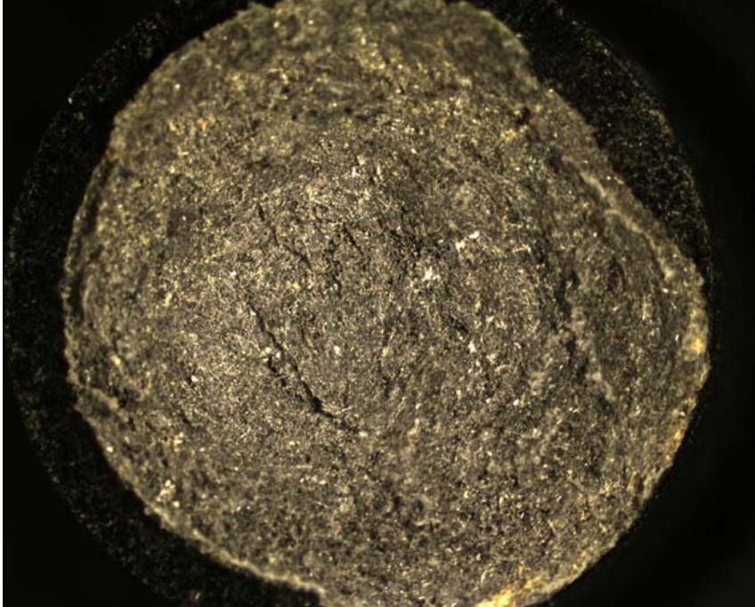
Figure F3: Sample 07-1091-B (head end) Fracture Surface As-Received
