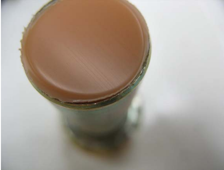
Figure D5: Cutting End of Cutter with Tap Slug
