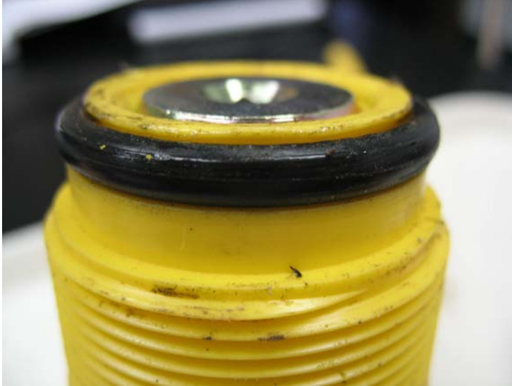
Figure D2: O-ring and Cutter Position in Tower with Cap Removed
