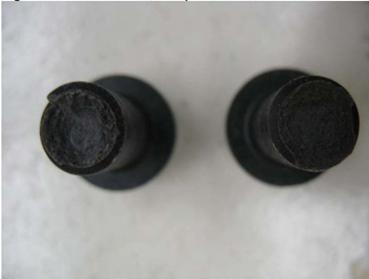
Figure D8: Broken Bolts, Sample 07-1091, Fracture Surfaces
