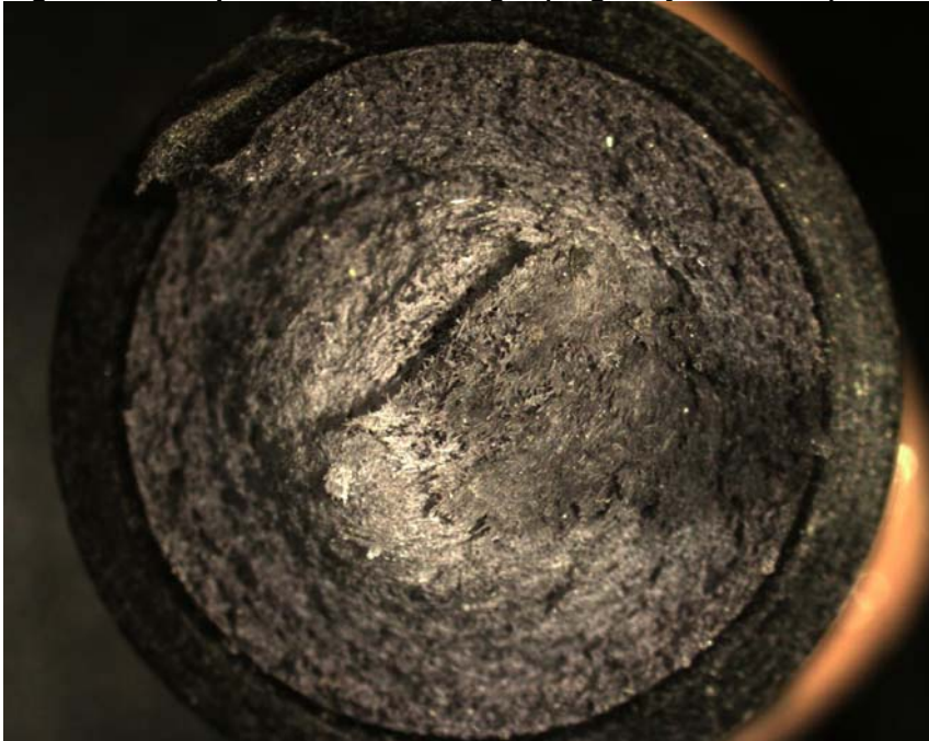
Figure F8: Sample 07-1090 Back Right (originally intact bolt) New Tensile Fracture Surface
