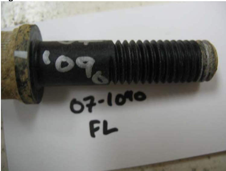
Figure D10: Front Left Intact Bolt
