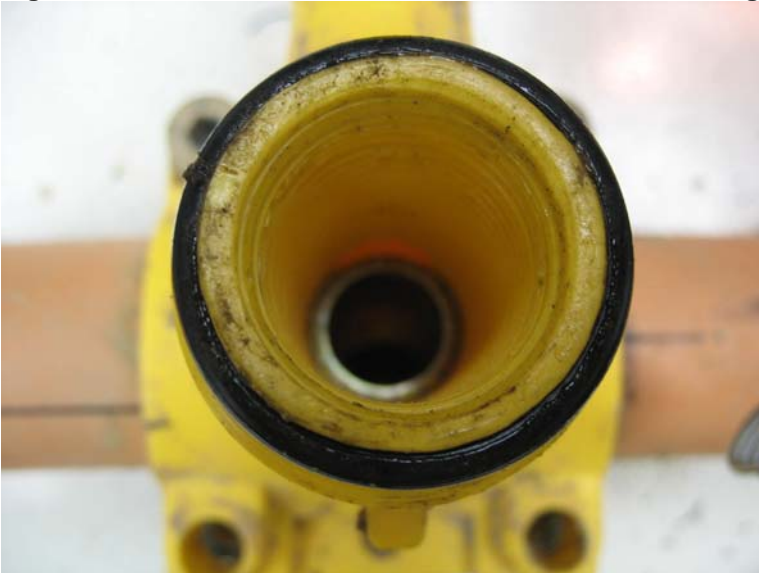
Figure D6: View Down Tower with Cutter Removed; Locking Sleeve at Bottom
