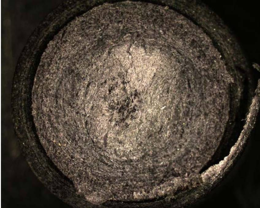
Figure F7: Sample 07-1090 Back Right New Fracture Surface After Tensile Testing
