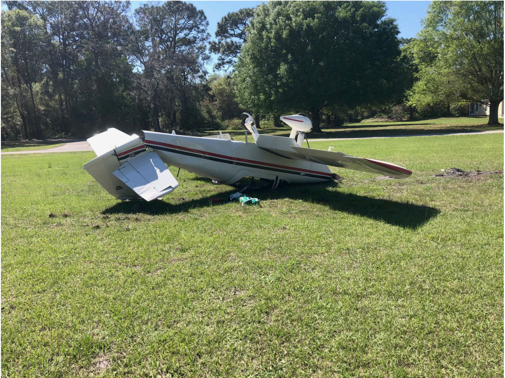
Photo 2 –View of airplane inverted on runway showing structural damage to fuselage.
