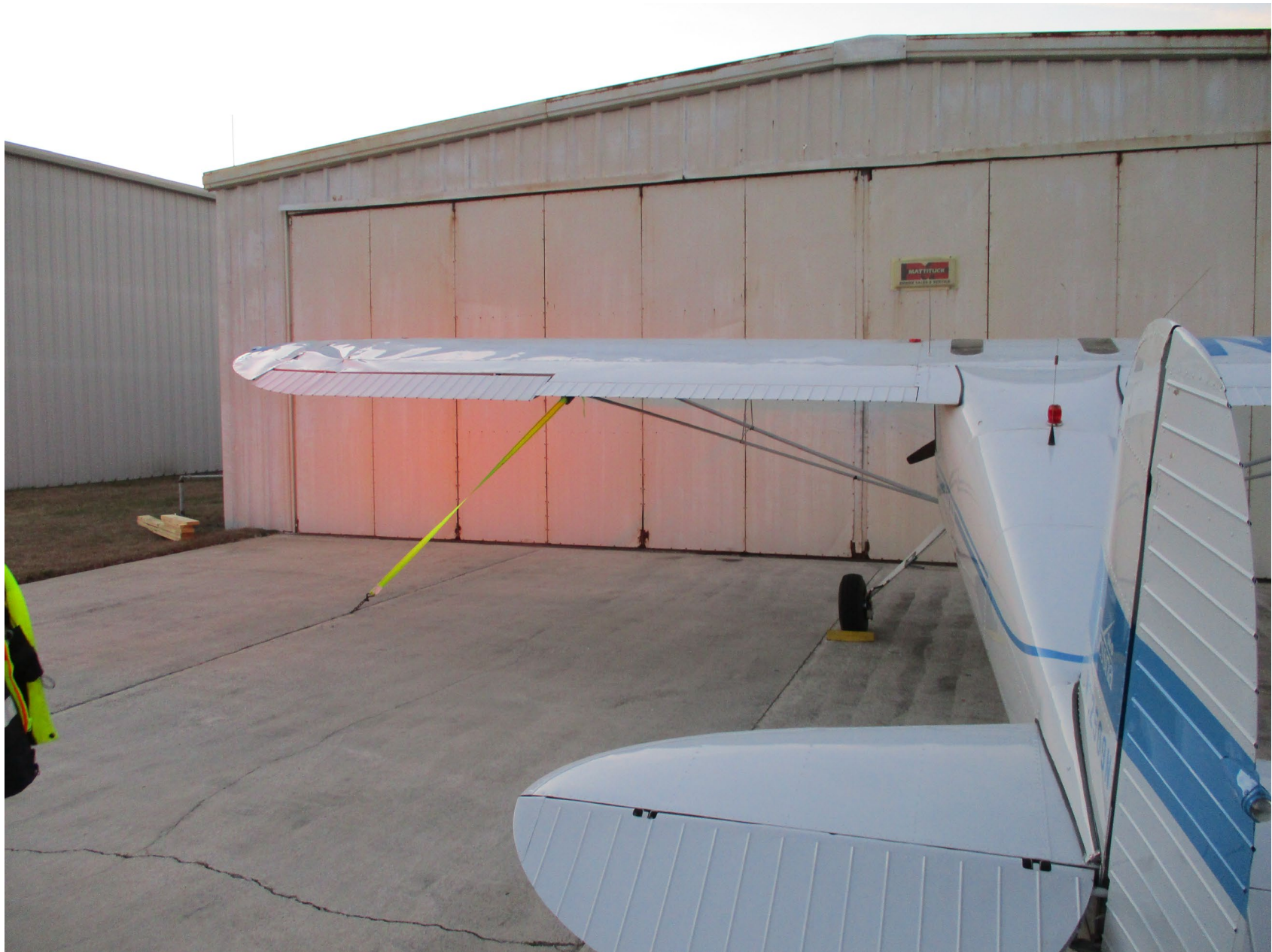
Photo 1 – View of left wing showing buckling damage on upper outboard section
