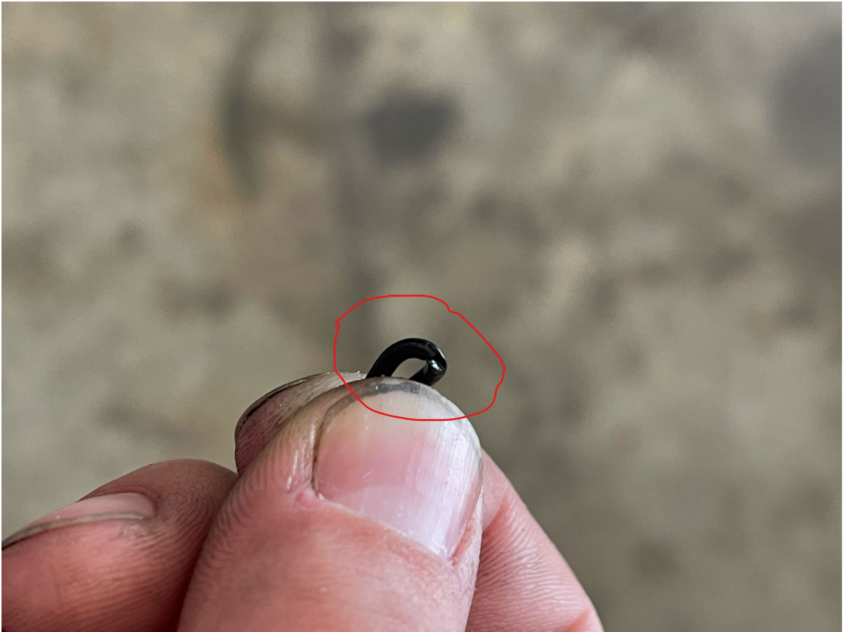
Photo 4 – Damaged O-ring showing pinch and cut
