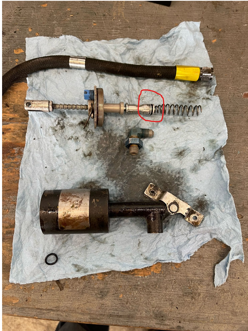
Photo 3 – Disassembled left brake master cylinder w/ damaged O-ring circled in red
