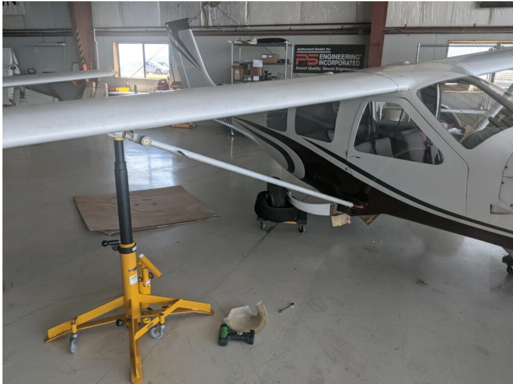
Photo 1 – Right main gear fractured (FAA)
