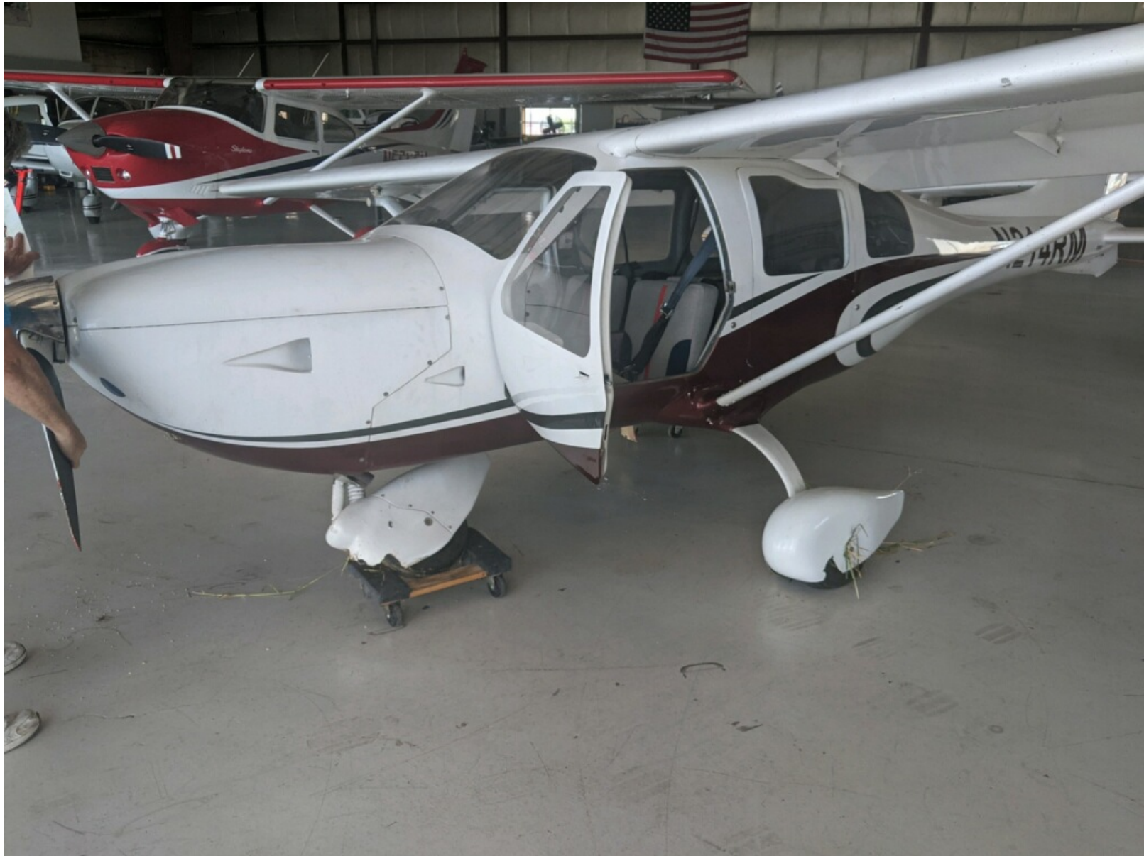
Photo 2 – Nose Gear Fractured (FAA)
