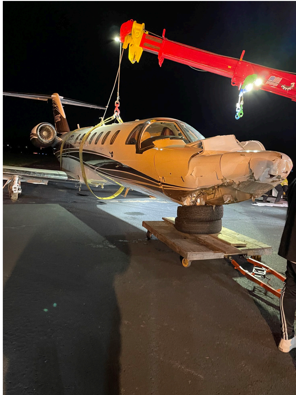
Photo 3 – View of the airplane after recovery from the ditch showing structural damage to the nose of the airplane.
