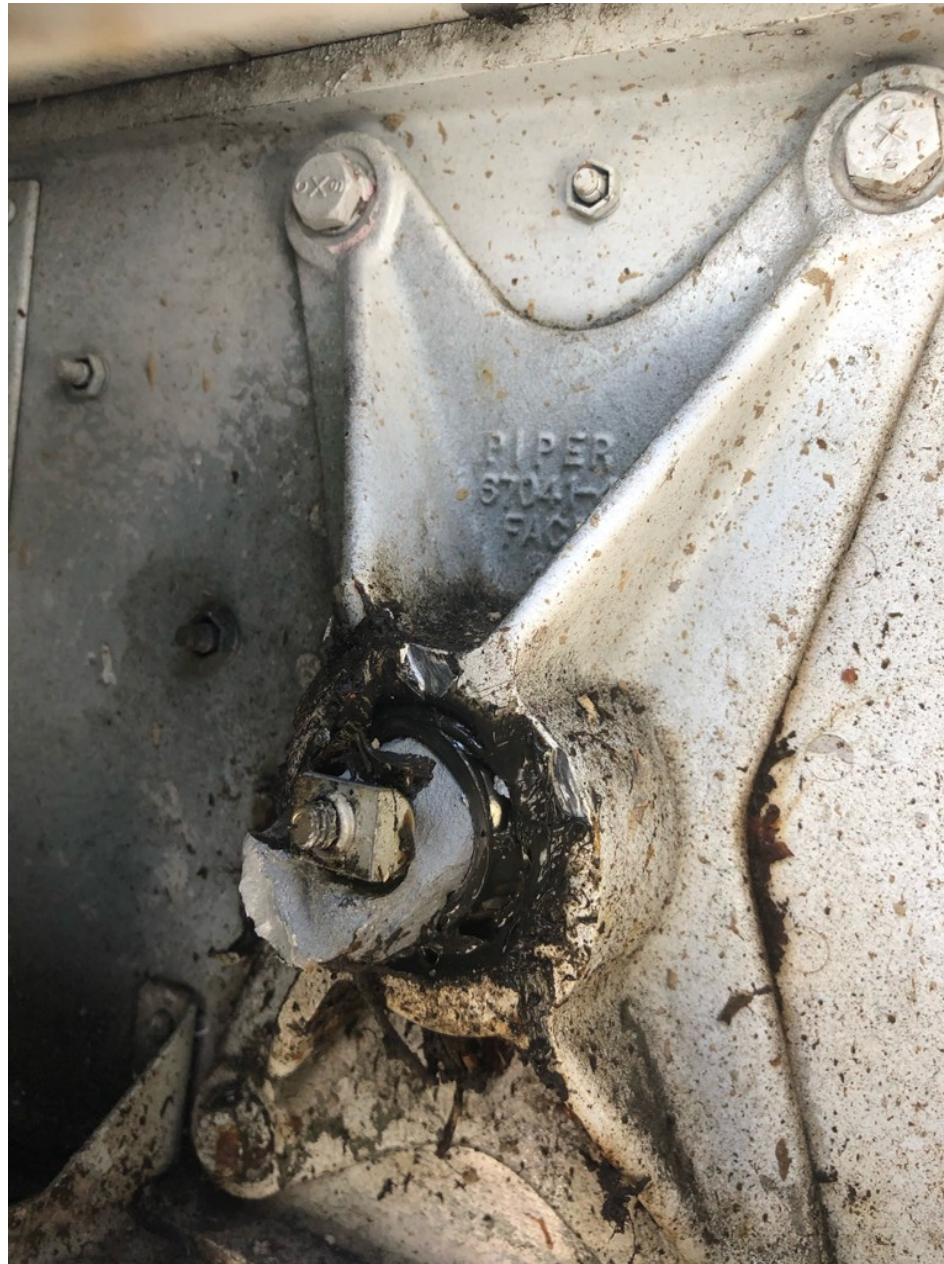
Photo 4 - Digital Photograph From Airport Manager. View Depicting the Fractured Left Trunnion and the Forward Trunnion Fitting.
