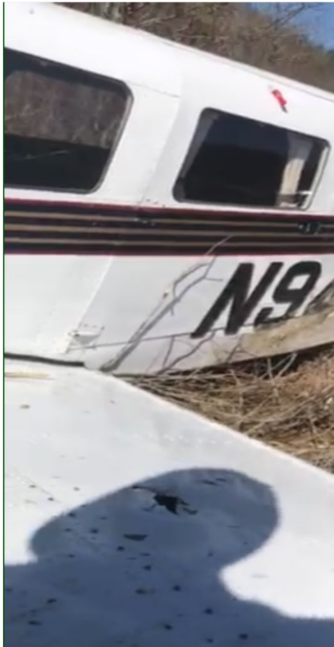
Photo 2 – Screen Shot from Video Taken After the Accident. View of the Upper Wing Skin of the Left Wing With a Hole Above the Location of the Trunnion in a Normally Installed Position.
