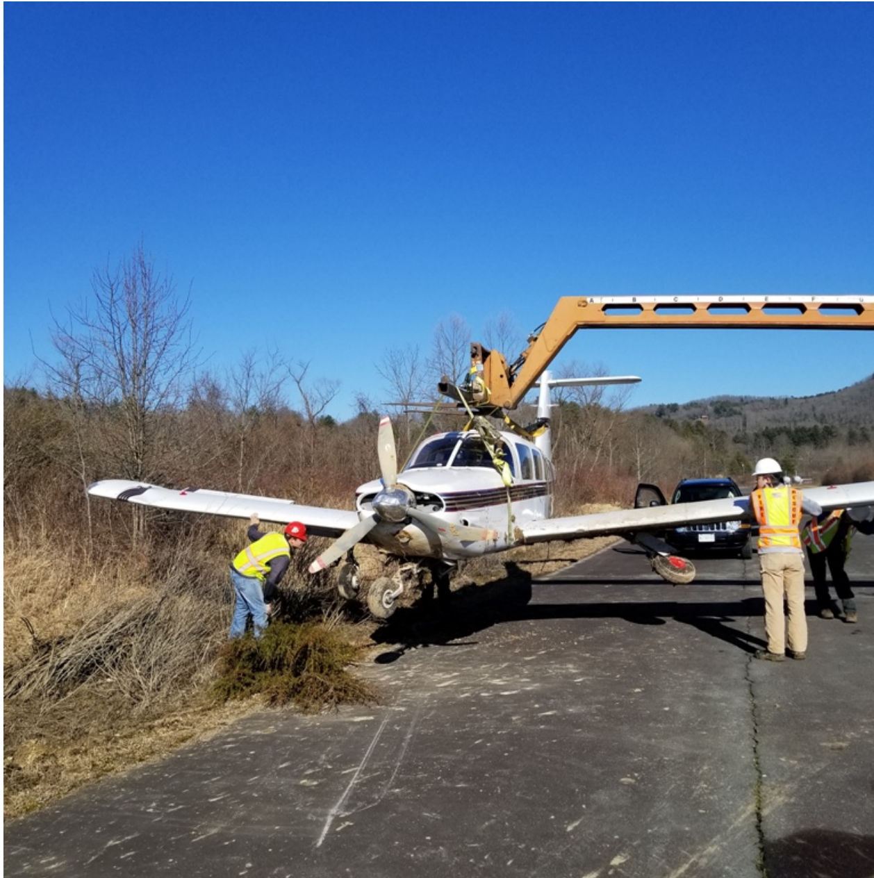
Photo 5 – FAA Digital Photograph. Forward View of the Airplane During Recovery. Note the Compression Wrinkle on the Upper Wing Skin of the Right Wing Just Outboard of the Fuel Cap.
