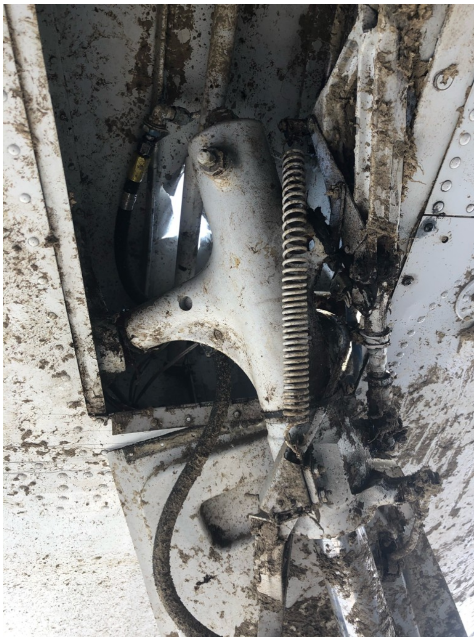
Photo 3 - Digital Photograph From Airport Manager. View Depicting the Displaced Left Main Landing Gear. Note the Hole Punctured in the Upwards Direction of the Upper Wing Skin.
