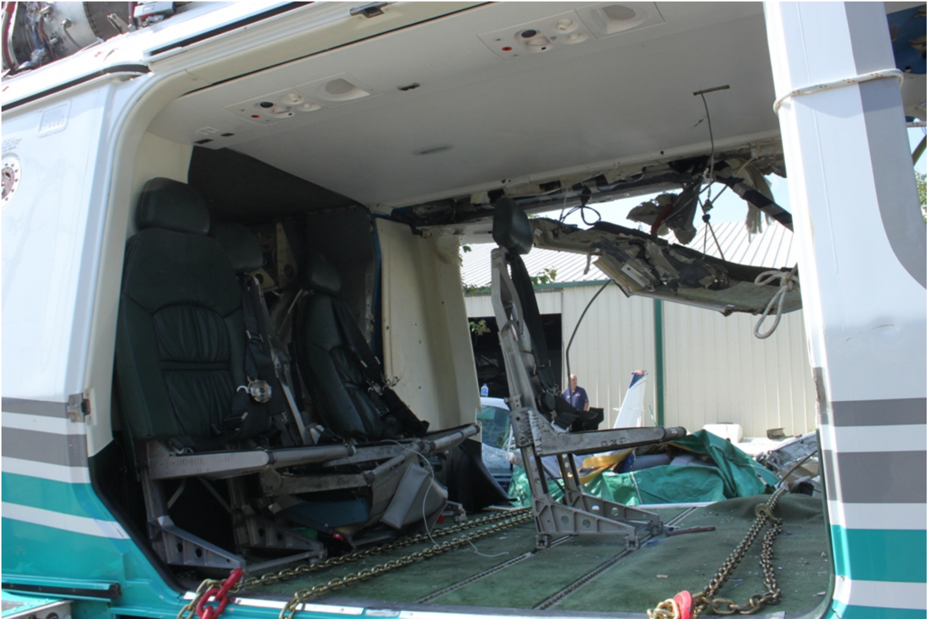
Photo 8 - NTSB Digital Photograph. Right Side View of the Aft Row Seats Remaining Installed Following Recovery.
