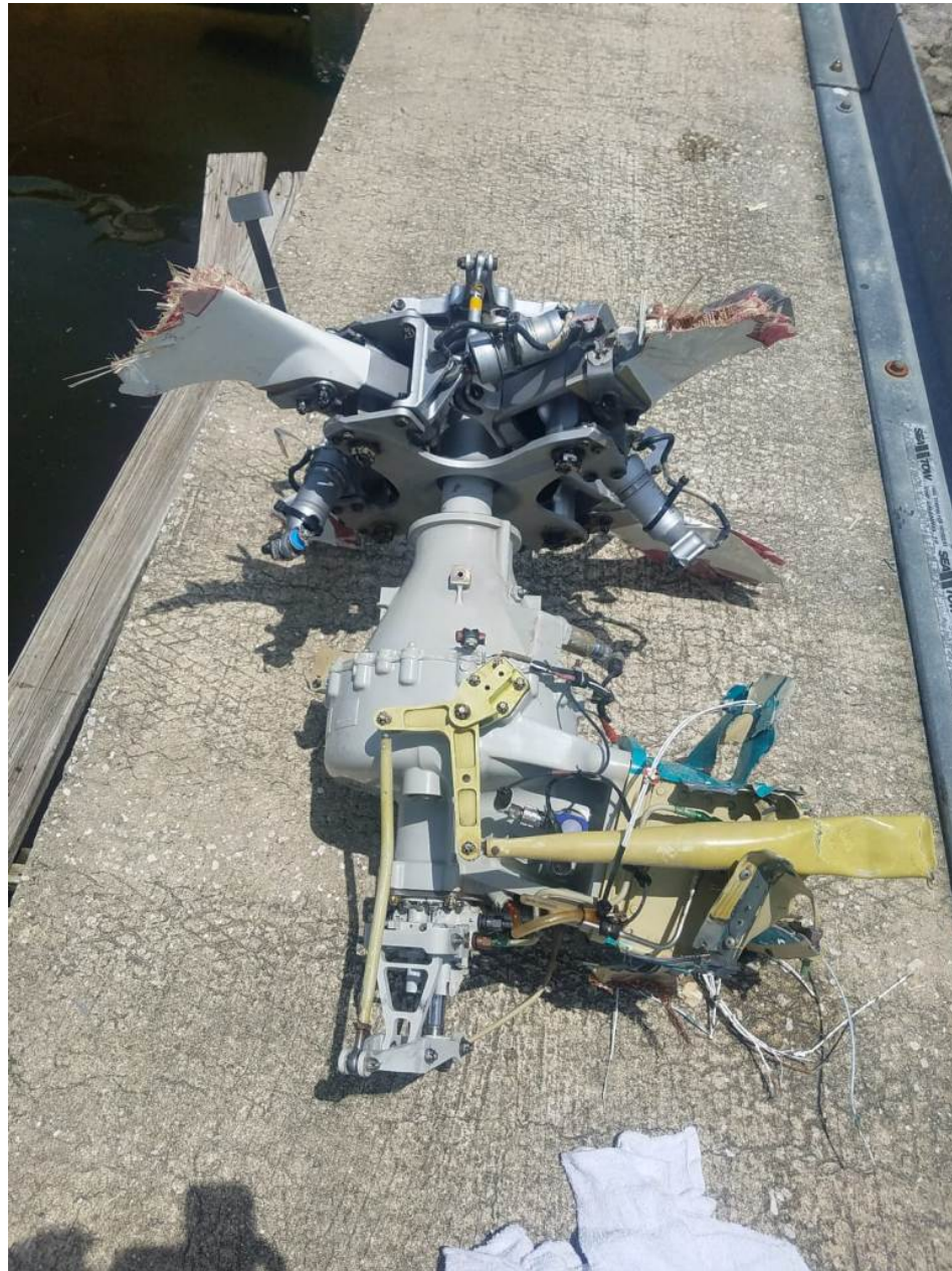
Photo 10 - Photograph Provided by Bahamian Accredited Representative. View of the Recovered Tail Rotor Assembly. Note the Fractured Tail Rotor Blades.
