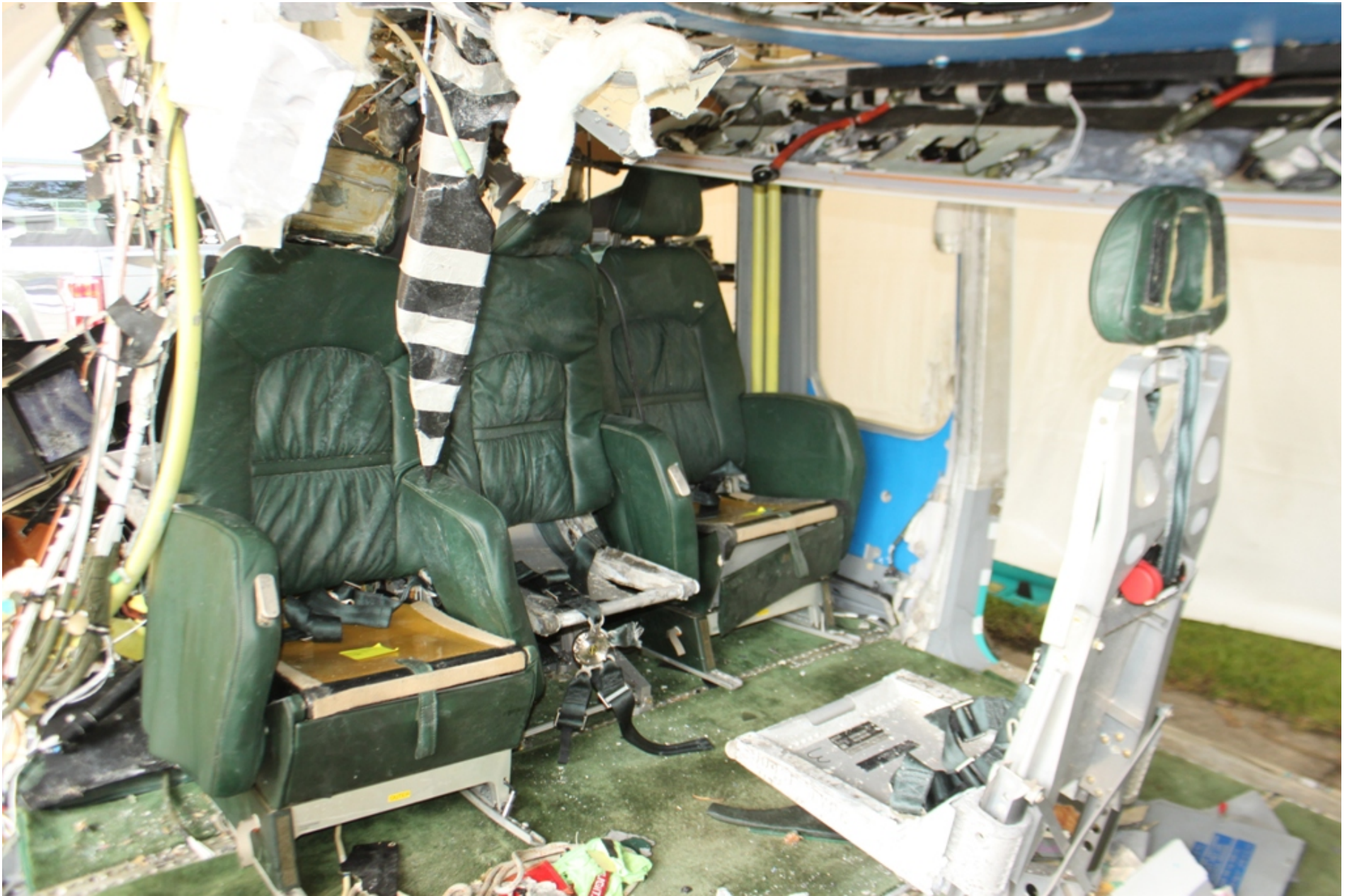
Photo 9 - NTSB Digital Photograph. Left Side View of the Middle Seat and Forward Row Seats Installed Following Recovery.
