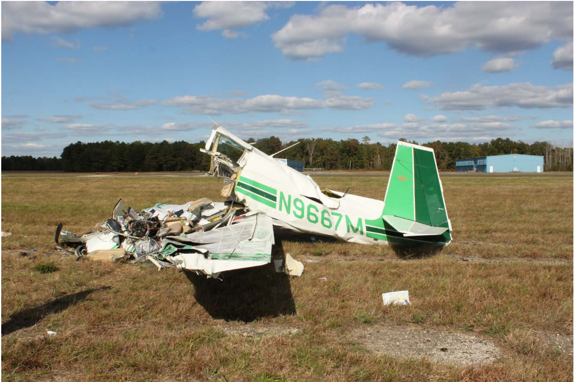
Photo 3 - NTSB Digital Photograph. Left Side View of the Airplane at the Accident Site. Note the destroyed Cockpit Area.
