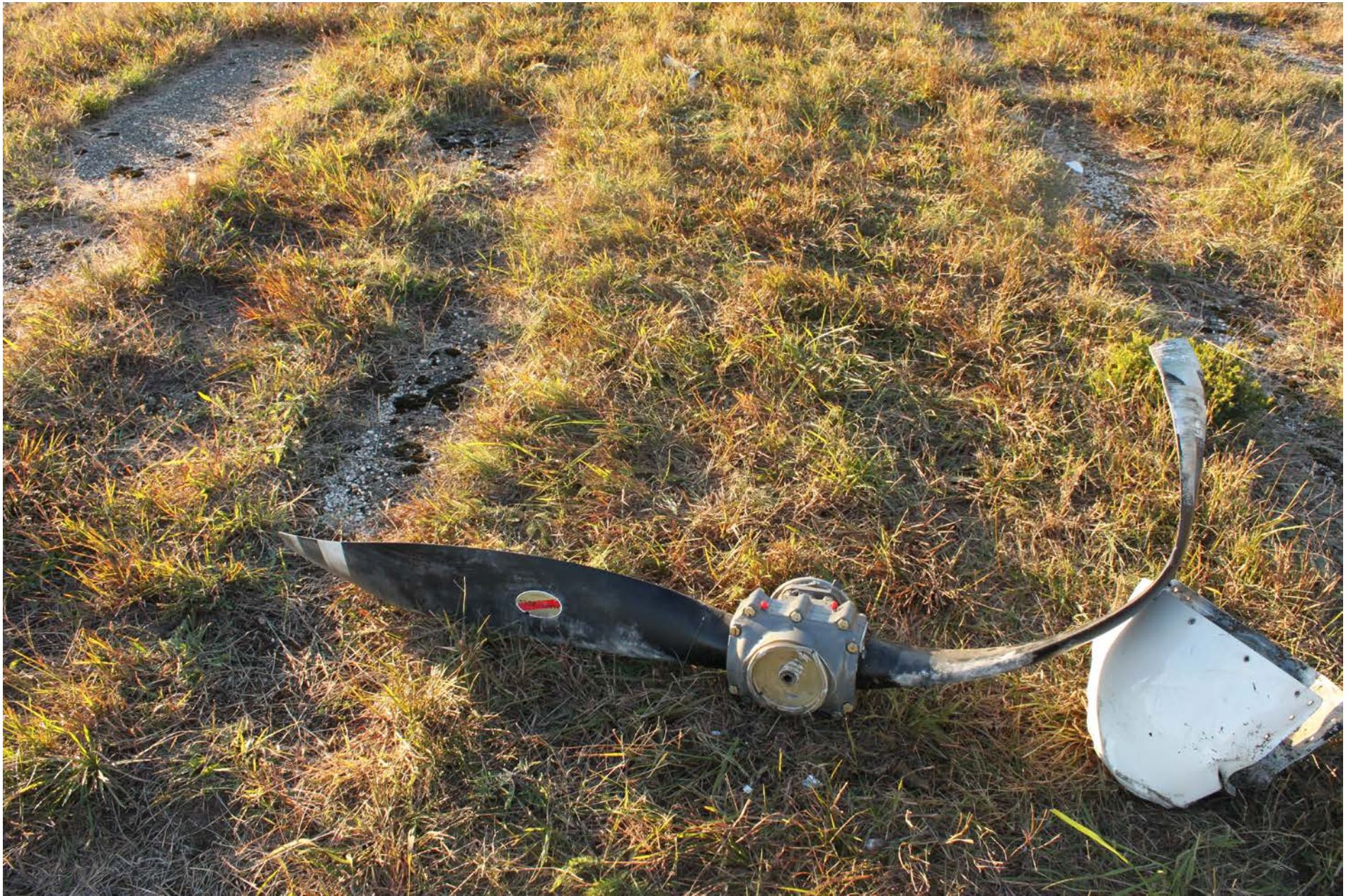
Photo 6 - NTSB Digital Photograph. View of the Separated Propeller at the Accident Site. Note the Blade Bending.
