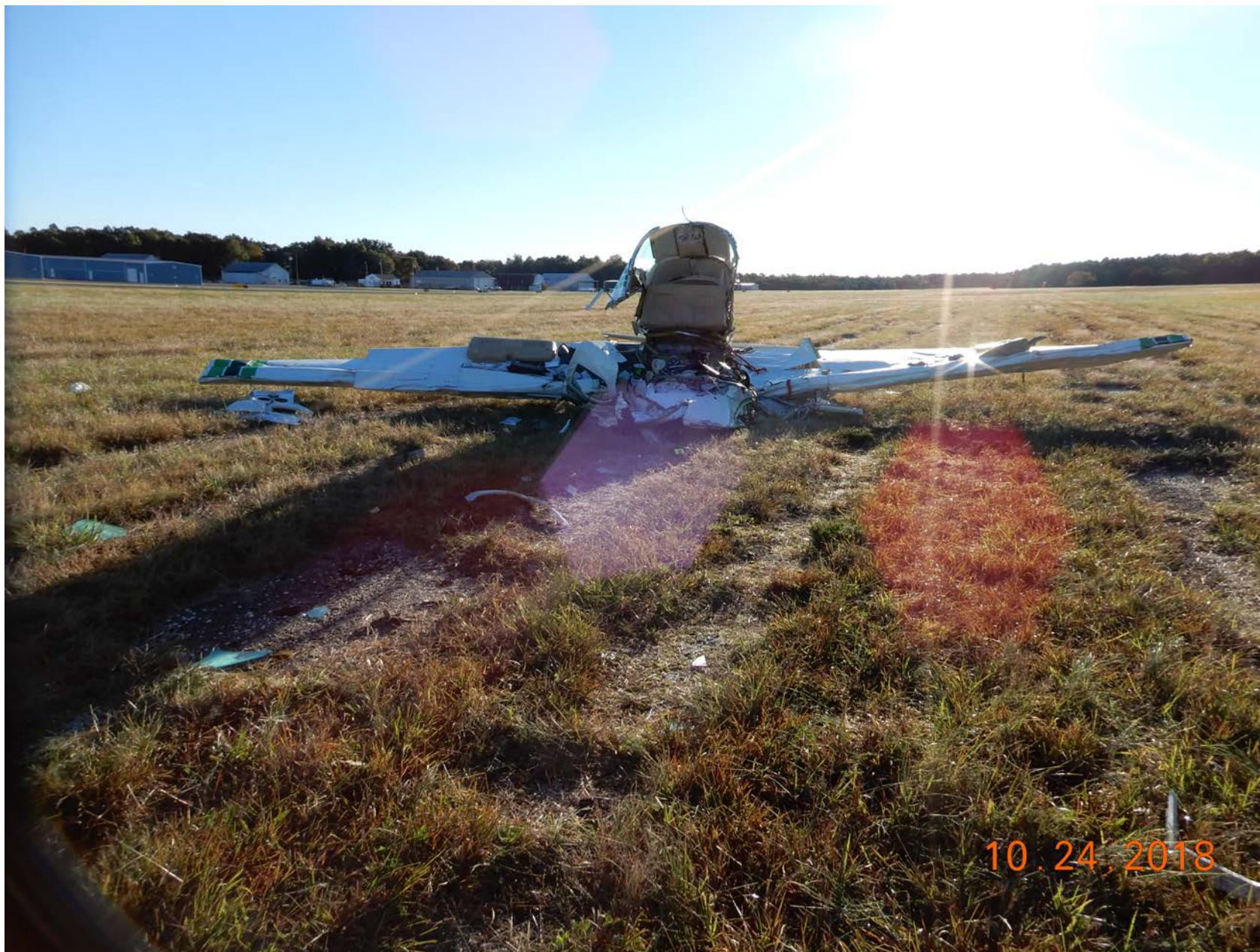
Photo 2 – NTSB Digital Photograph. Frontal View of the Airplane at the Accident Site. Note the Deformation to the Leading Edges of Both Wings.
