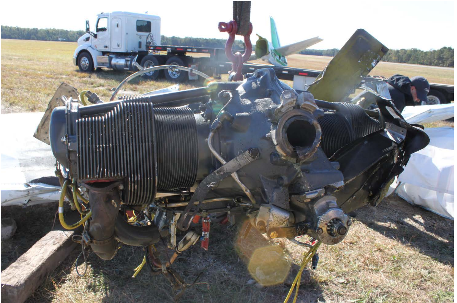
Photo 7 - NTSB Digital Photograph. Frontal View of the Engine at the Accident Site. Note the Fractured Crankshaft.
