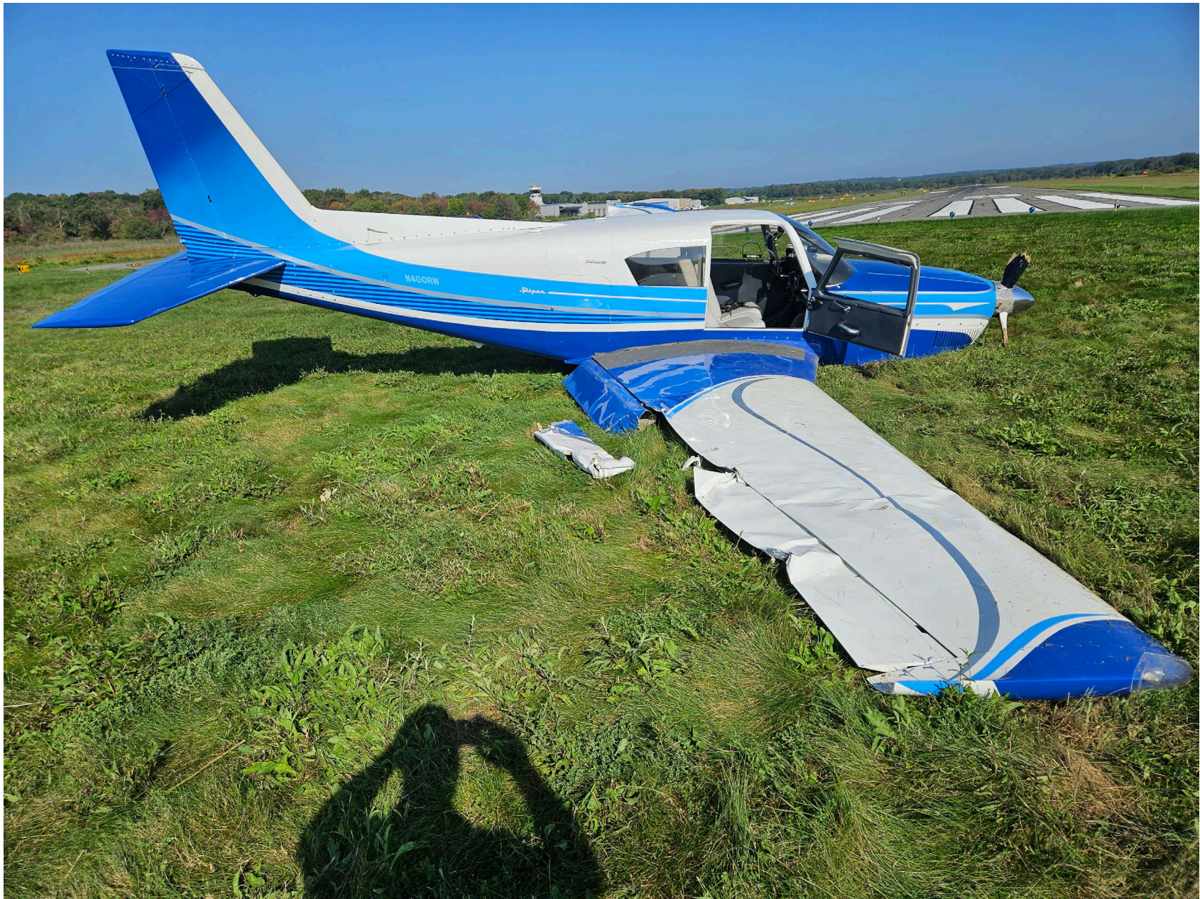
Photo 1 – Digital Photograph From Airport Manager. Right Side View of the Airplane where it Came to Rest. Note the Proximity to the Runway in the Background and the Structural Damage to the Right Wing.
