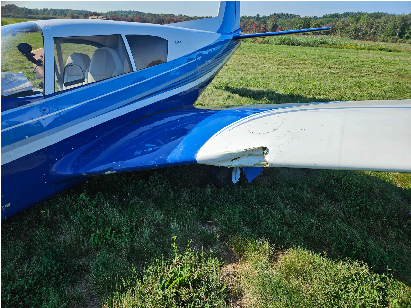
Photo 3 - Digital Photograph From Airport Manager. View of the Inboard Portion of Left Wing and Left Side of a Portion of the Fuselage. Note the impact Damage on the Leading Edge of the Left Wing Near the Wing Root.
