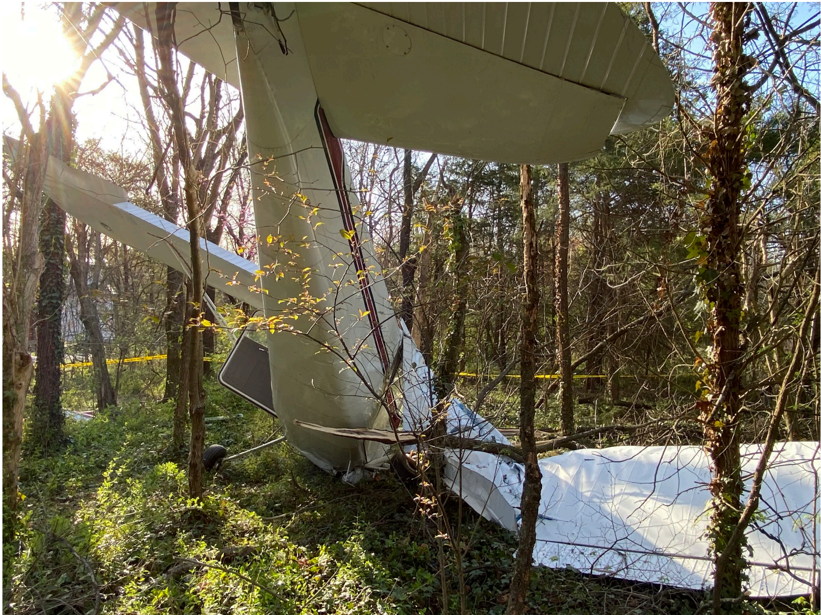
Photo 2 - FAA Digital Photograph. Right Rear View of the Airplane at the Accident Site. Note the Structural Damage to the Right Wing.
