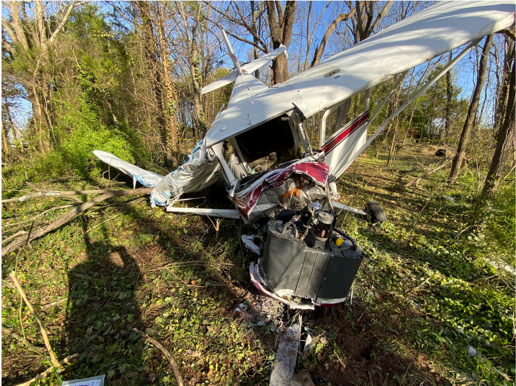
Photo 3 - FAA Digital Photograph. Frontal View of the Airplane at the Accident Site Depicting Nearly the Entire Airframe Except Outer Portion of the Left Wing. Note the Structural Damage to the Right Wing.
