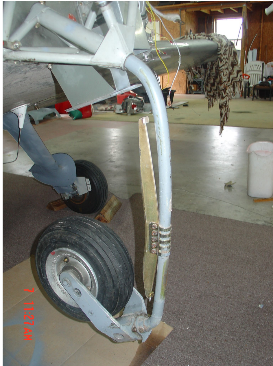
Photo 4 - Digital Photograph Provided by Owner/Pilot. Right Side View of the Nose Landing Gear Following Recovery of the Airplane. Note the Aft Displacement of the Nose Gear Leg.
