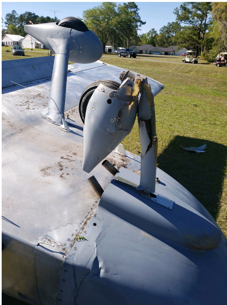
Photo 3 - Digital Photograph Provided by FAA. Left Side View of the Inverted Airplane At the Accident Site, and the Nose and Right Main Landing Gears visible. Note the Aft Displaced Nose Landing Gear.
