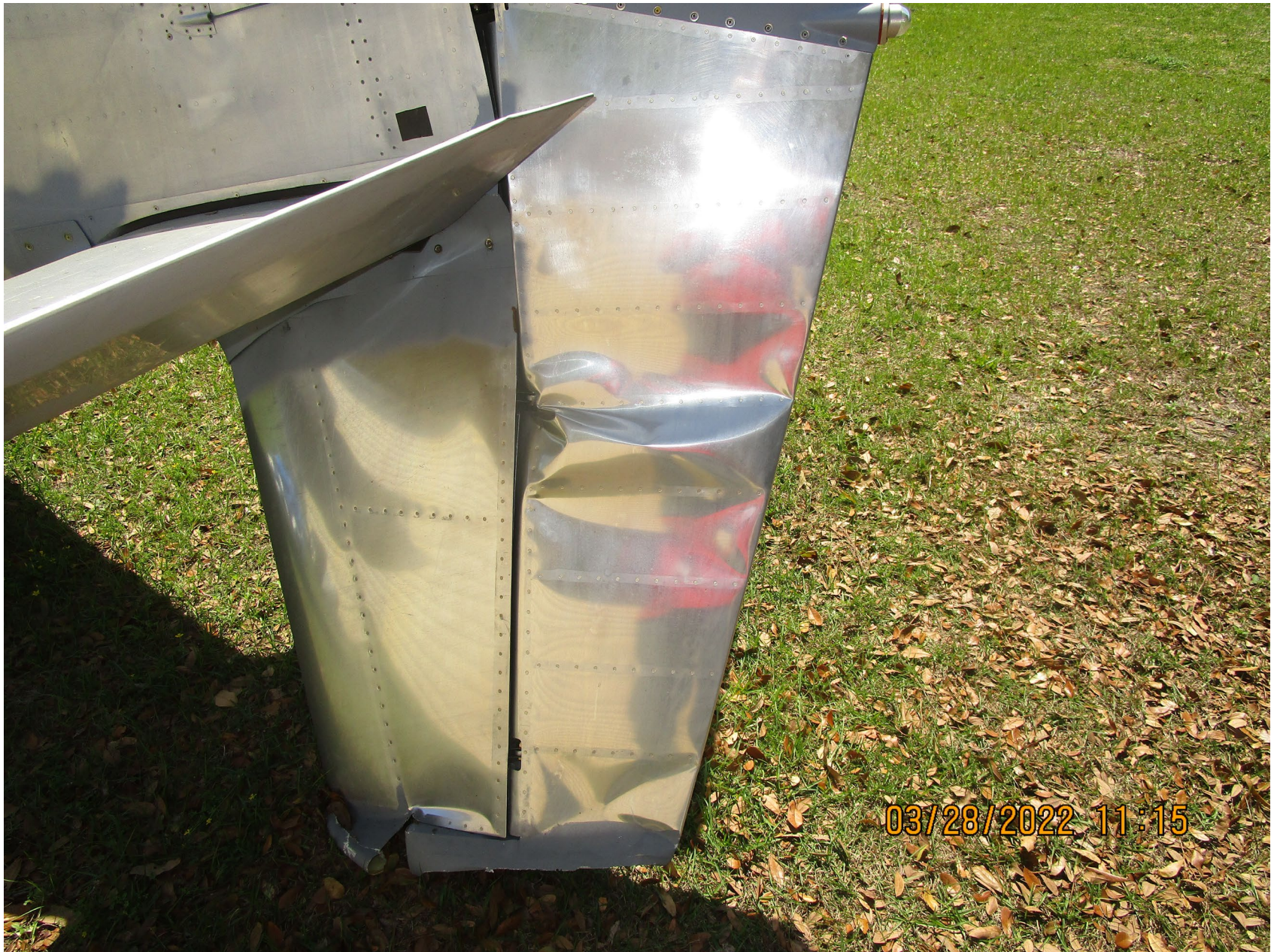
Photo 2 - Digital Photograph Provided by FAA. View Depicting the Substantial Damage to the Rudder Flight Control Surface.
