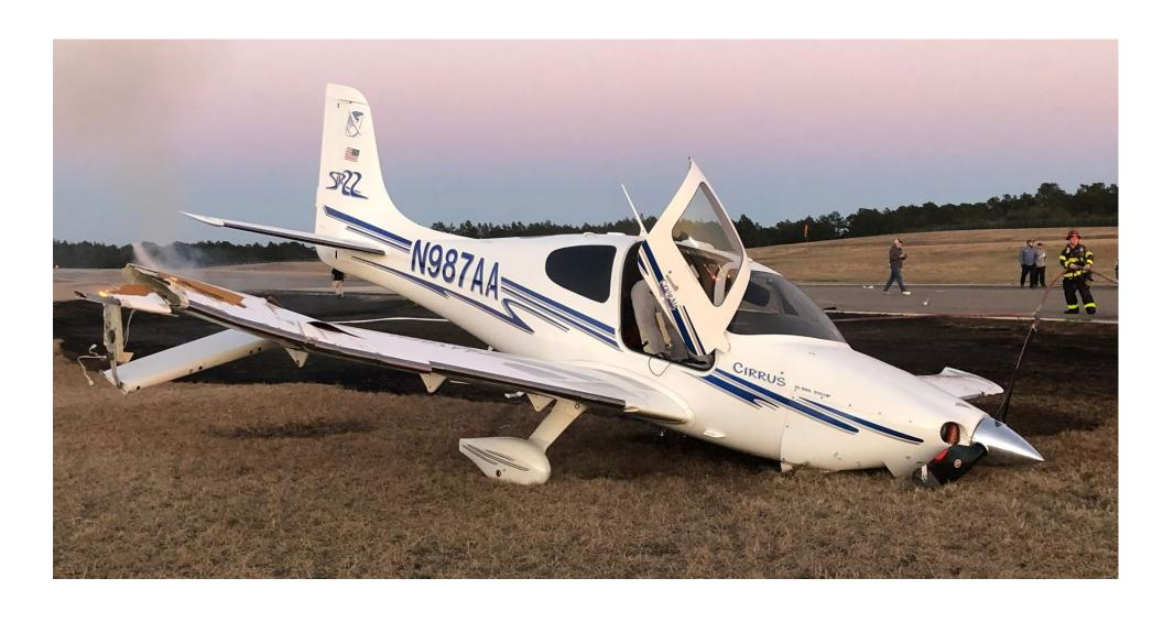
Photo 1 – Digital Photograph From Insurance Adjuster. Right Forward Quartering View of the Airplane Depicting the Right Side of the Airplane, and Structural Damage to the Right Wing.
