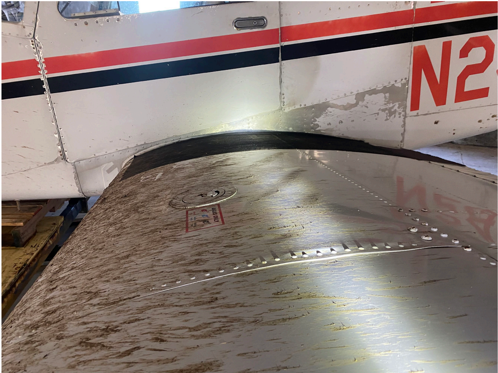
Photo 2 - FAA Digital Photograph. View Depicting the Wrinkles in the Upper Skin of the Left Wing.
