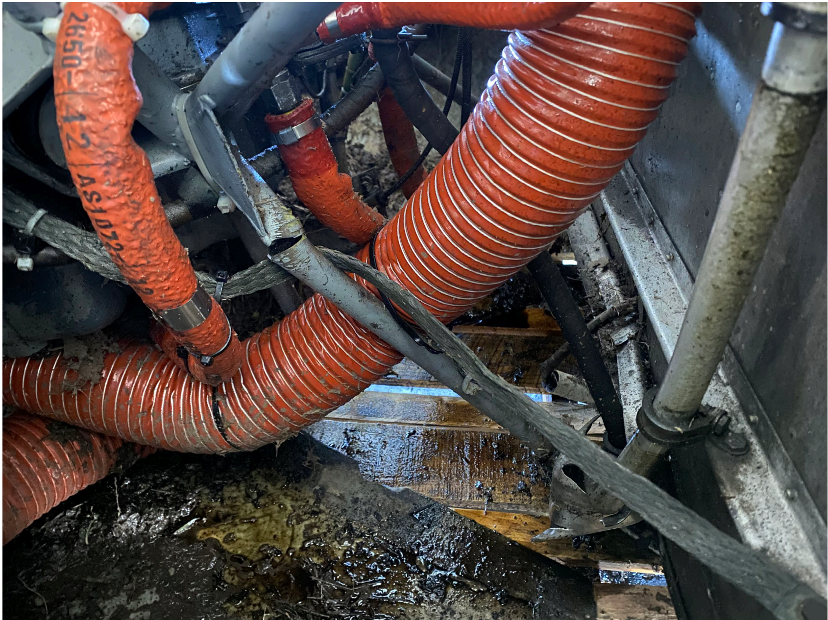
Photo 1 – FAA Digital Photograph. View of a fractured Engine Mount Tube.
