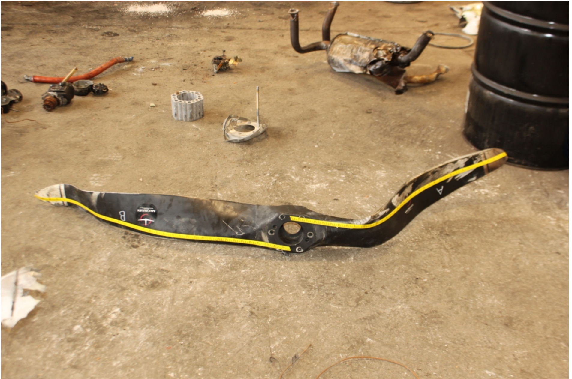
Photo 12 - NTSB Digital Photograph. View of the Propeller Following Separation From the Engine During Follow-Up Examination. Note the “S” Type Blade Bending of Both Blades.
