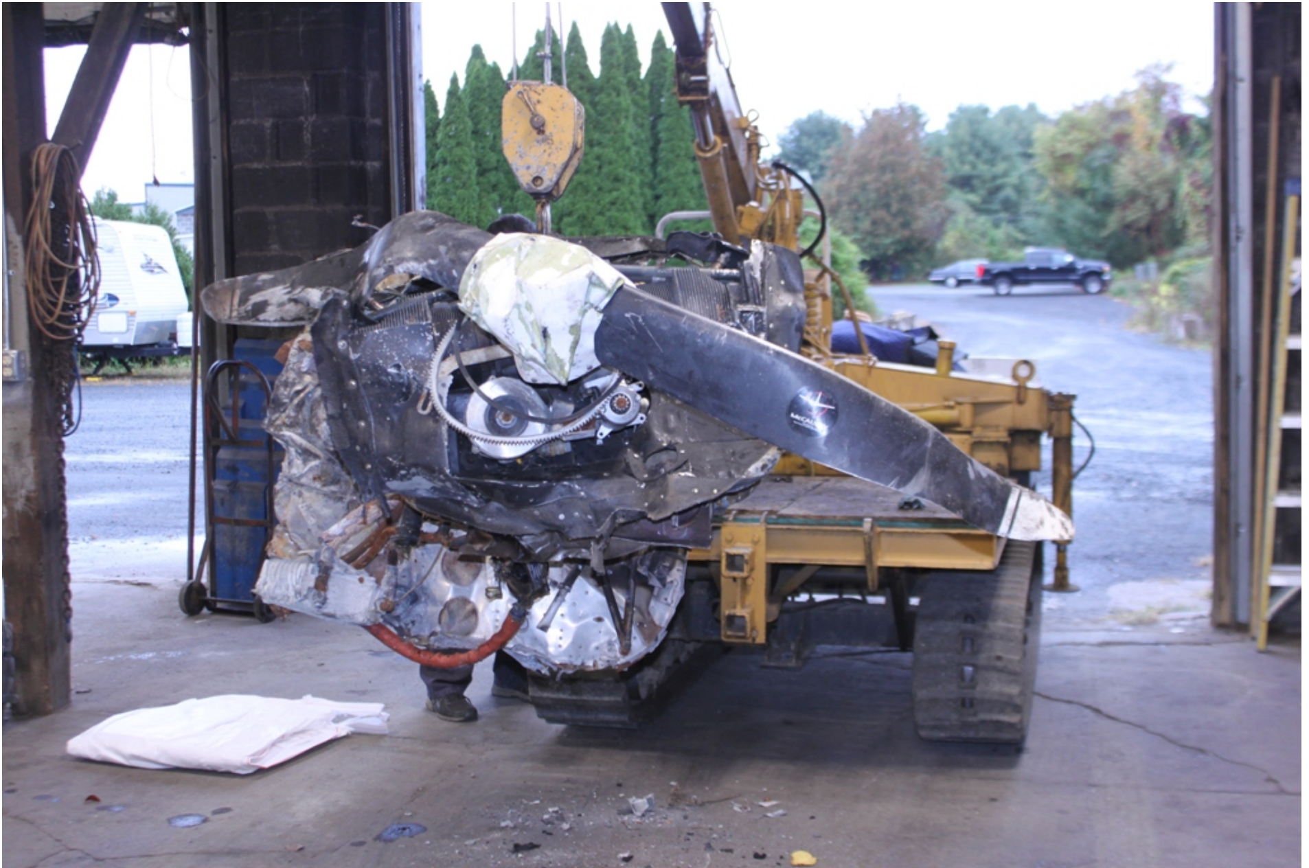
Photo 11 - NTSB Digital Photograph. Frontal View of the Engine Assembly with Attached Propeller During Follow-Up Examination. Note the Propeller Blade Bending.
