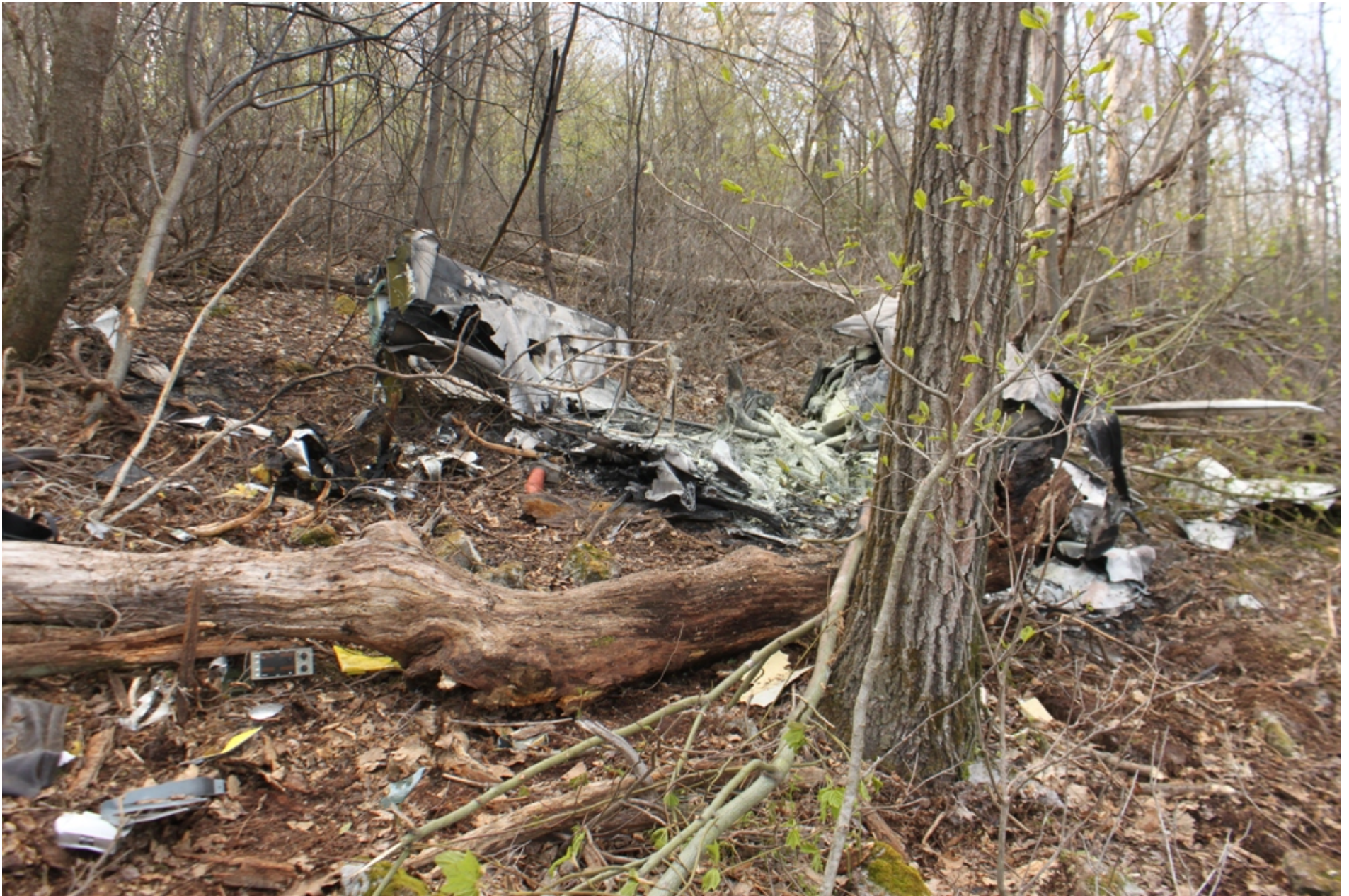
Photo 5 - NTSB Digital Photograph. View Depicting the Resting Position of the Main Wreckage Including the Cockpit Section, Engine Assembly.
