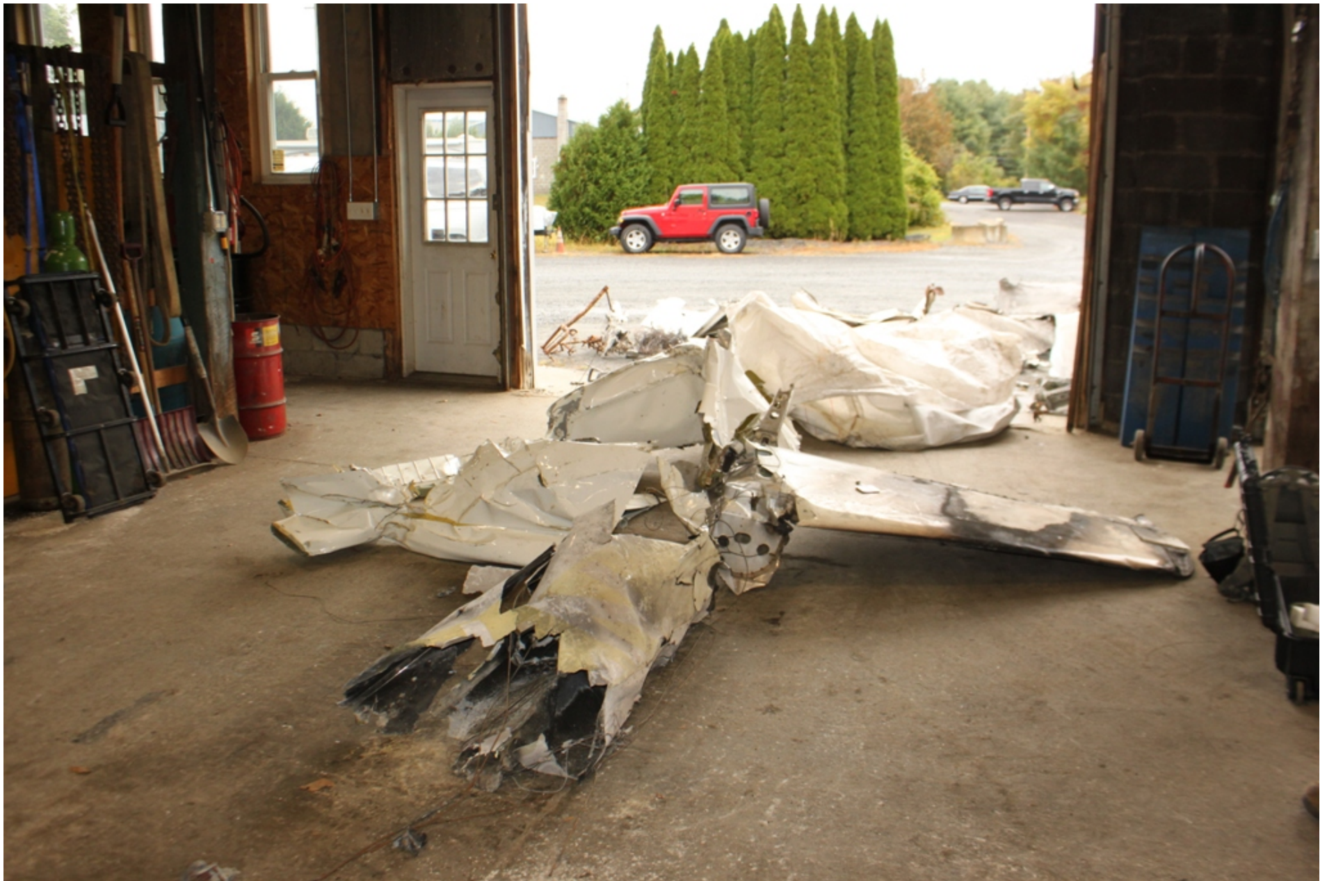
Photo 9 - NTSB Digital Photograph. View of the Aft Empennage Taken During Follow-Up Examination. Note the Extensive Fire Damage to the Fuselage Forward of the Attached Left Horizontal Stabilizer.
