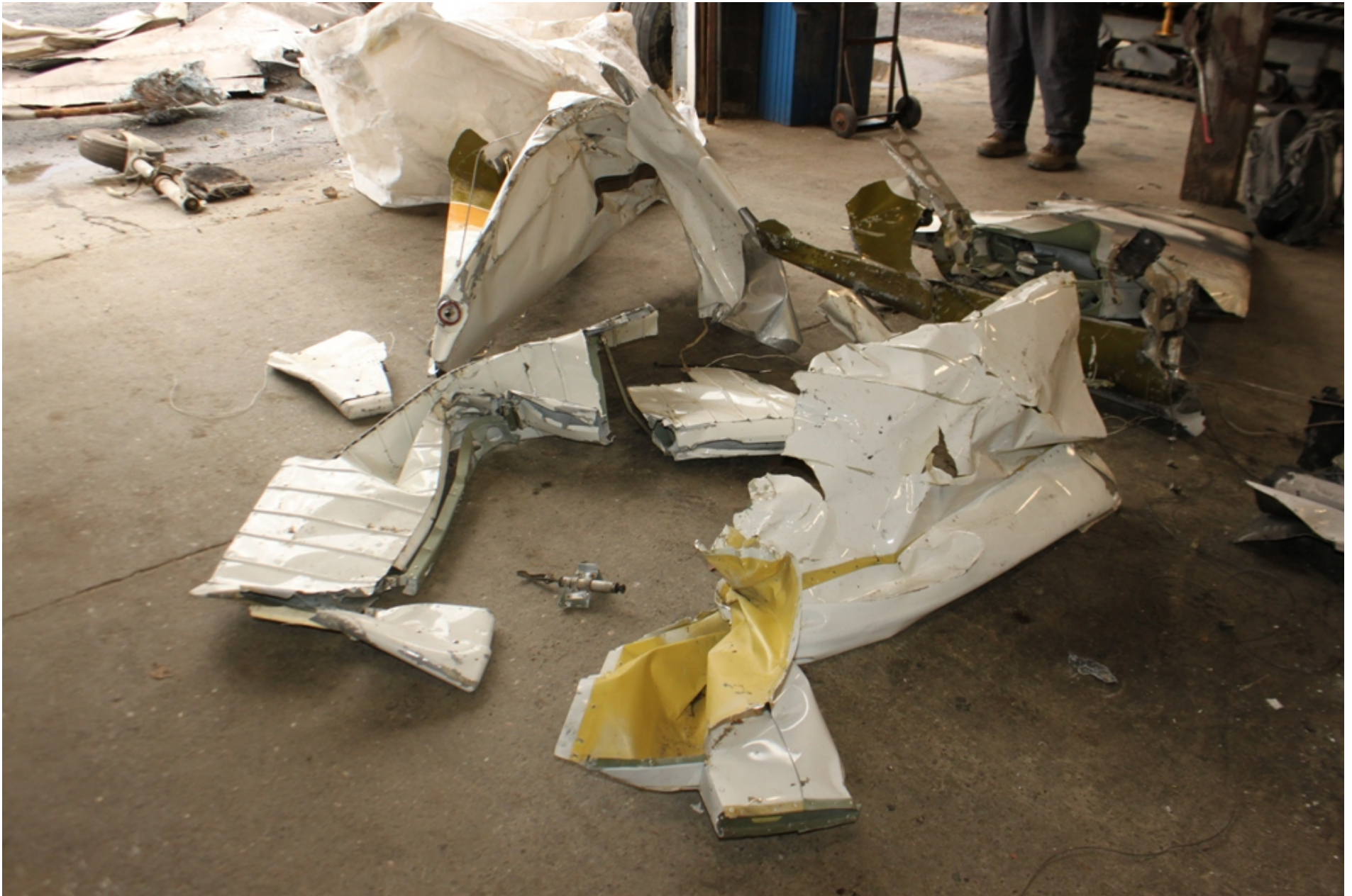
Photo 10 - NTSB Digital Photograph. View of the Separated Right Horizontal Stabilizer and Elevator Taken During Follow-Up Examination.
