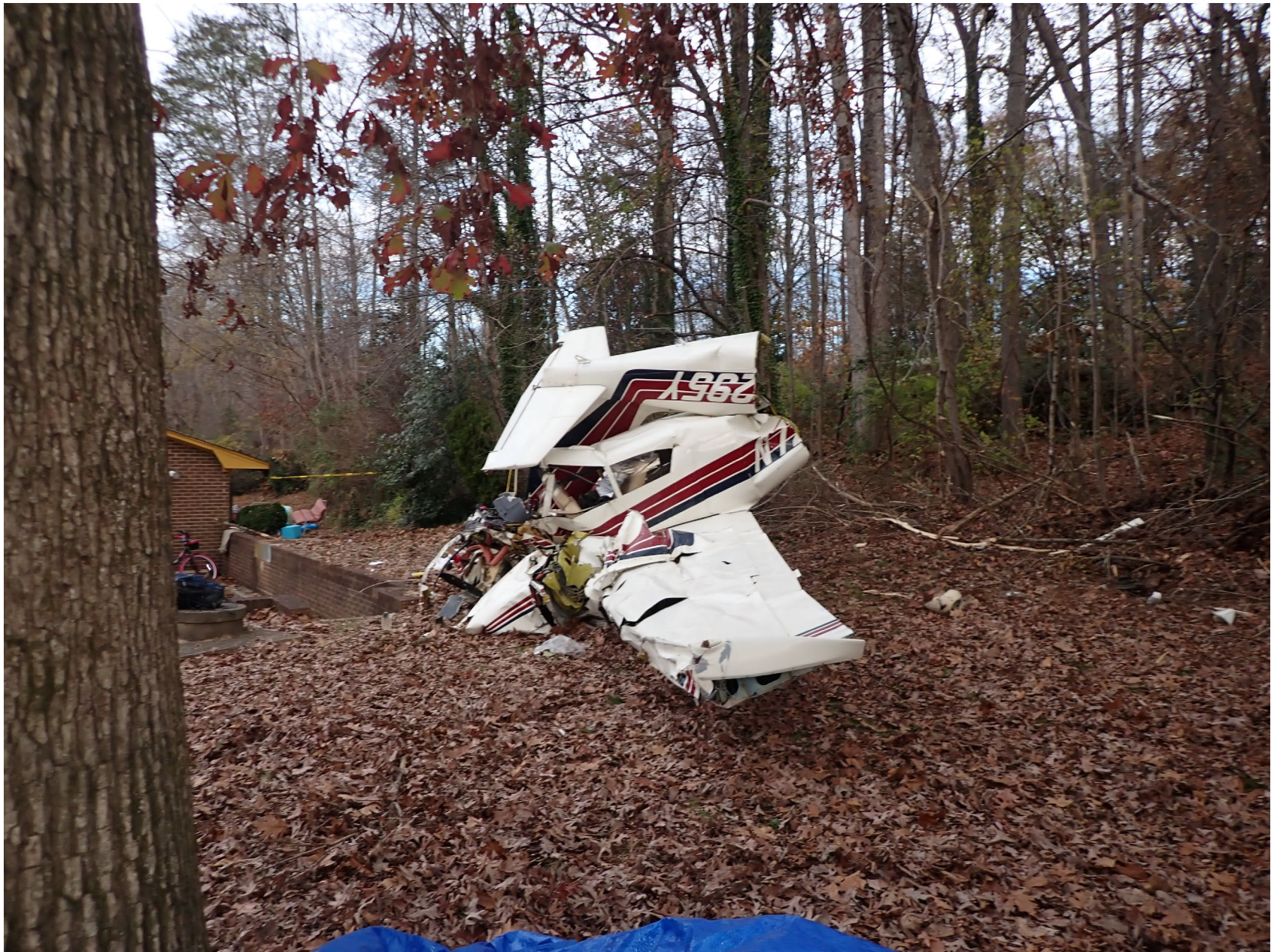
Photo 2 - NTSB Digital Photograph. Left Side View of the Wreckage at the Accident Site. Note the Aft Empennage Resting on Top of the Fuselage and Also Displaced to the Right.
