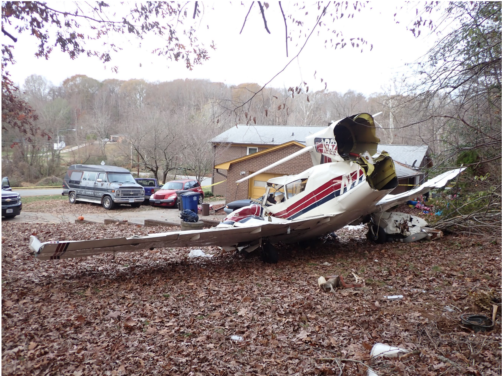
Photo 3 - NTSB Digital Photograph. Left Rear Quartering View of the Wreckage at the Accident Site. Note the Aft Empennage Resting on Top of the Fuselage and Also Displaced to the Right.
