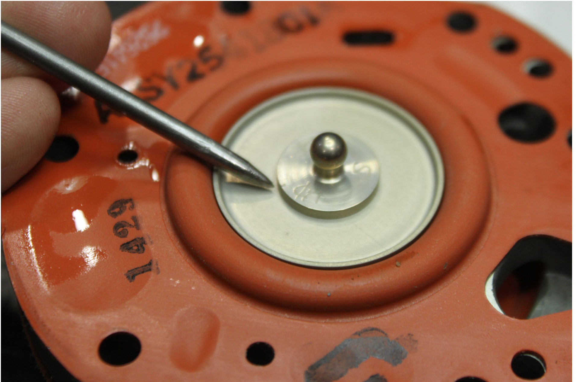
Photo 15 – NTSB Digital Photograph. Pointer is Pointing to Spec of Material on the Fuel Diaphragm of the Right Fuel Injection Servo.
