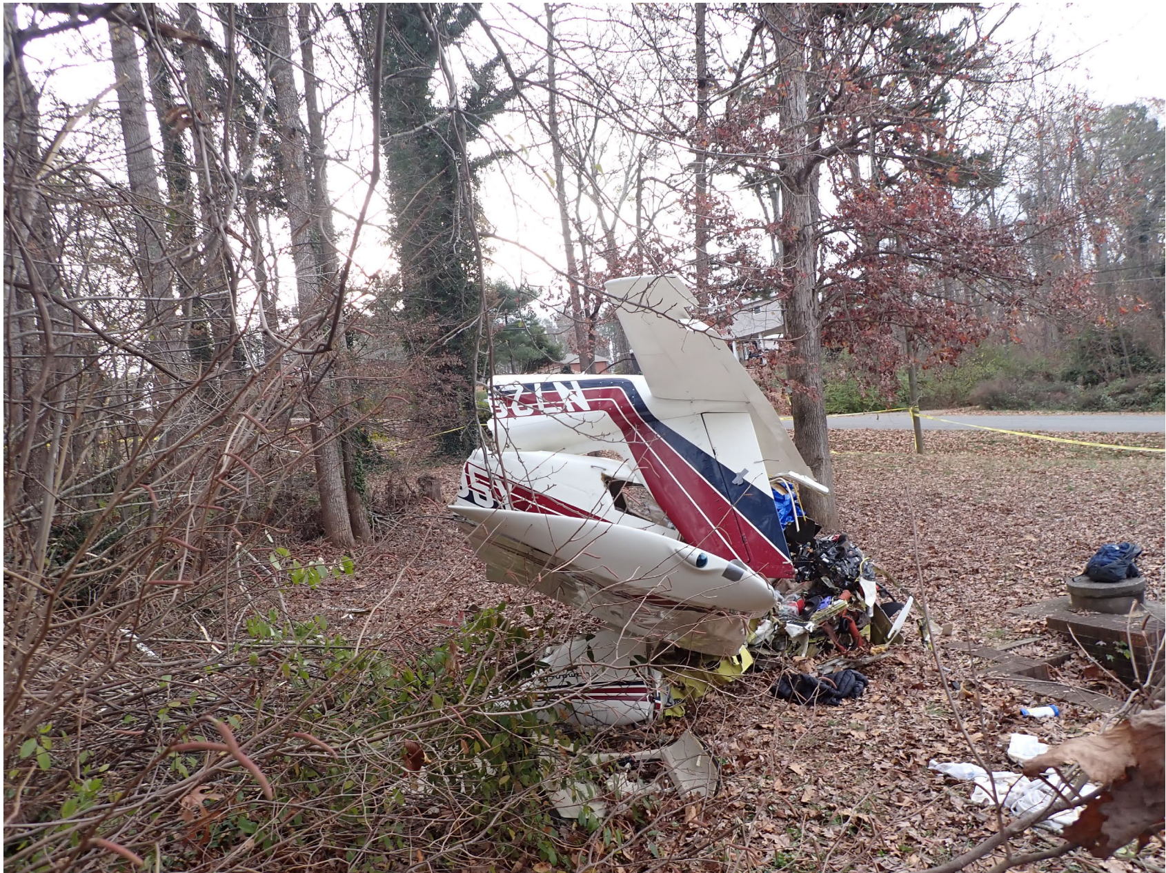
Photo 5 - NTSB Digital Photograph. Right Side View of the Wreckage at the Accident Site. Note the Aft Empennage Resting on Top of the Fuselage and Also Displaced to the Right.
