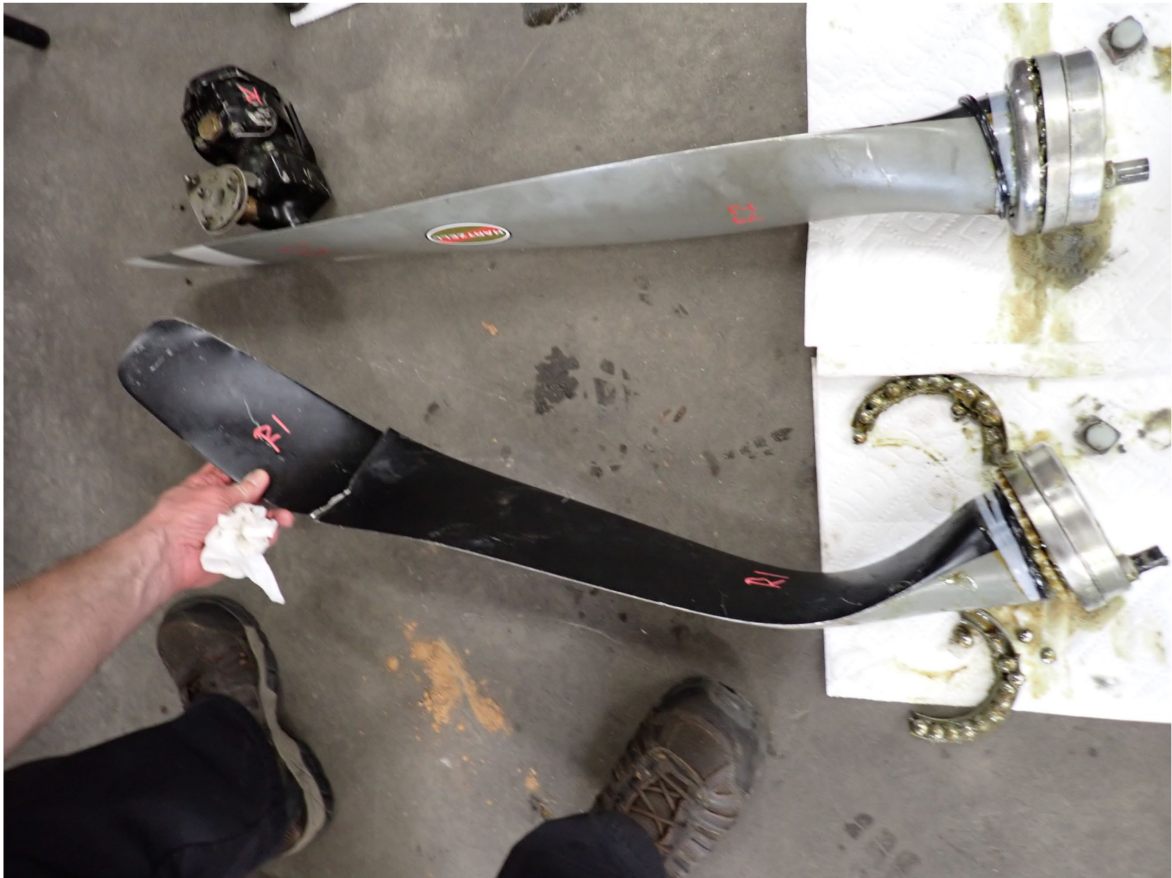
Photo 10 – Hartzell Digital Photograph. View of Both Right Propeller Blades Following Removal from the Hub and Also Right Propeller Governor. Note the R1 Blade Cut near the Tip For Recovery.
