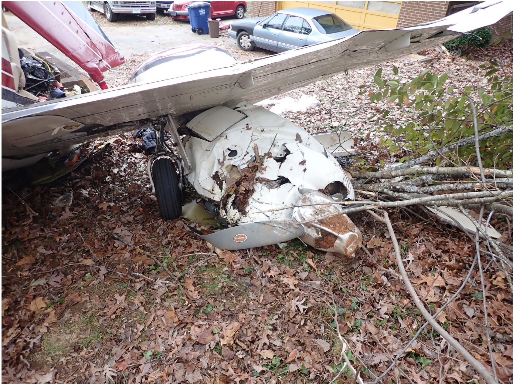
Photo 7 – NTSB Digital Photograph. View of the Resting Position of the Right Engine Assembly with Attached Propeller Assembly.
