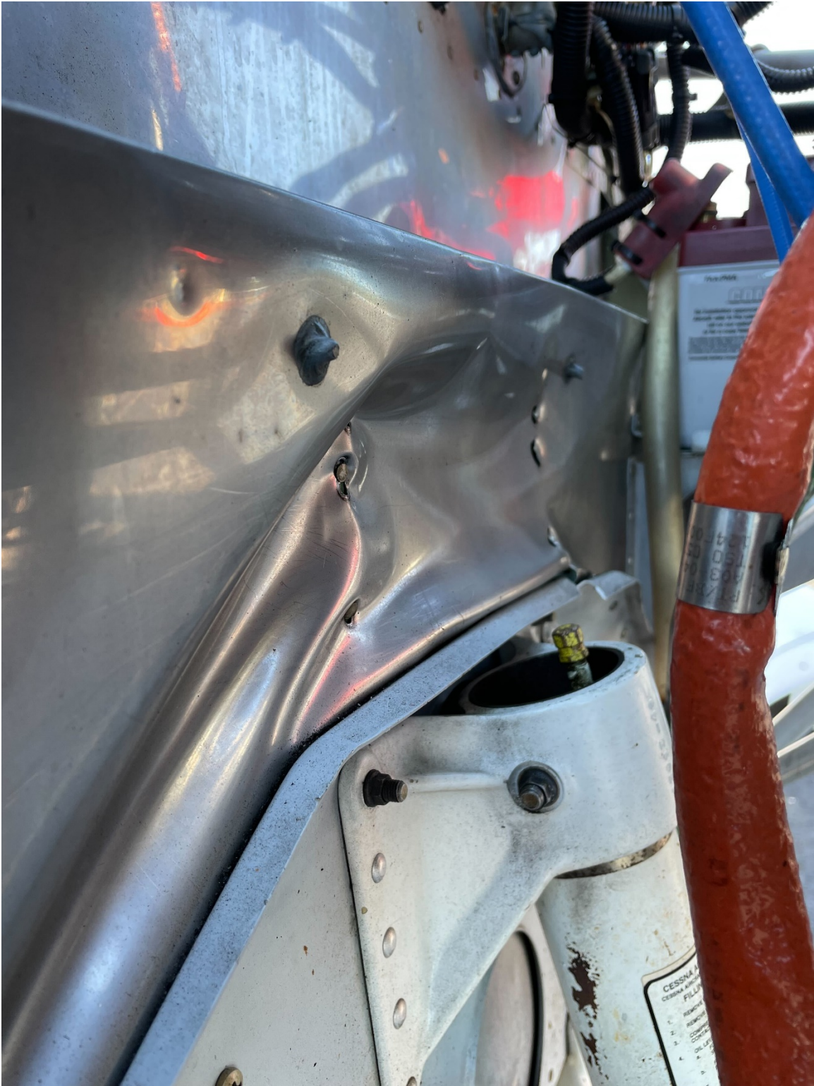
Photograph 2 – Accident airplane – Firewall damage.
