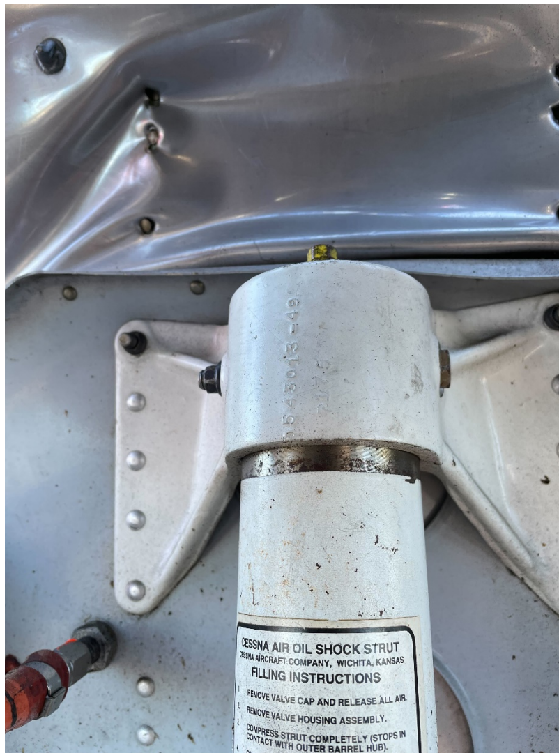
Photograph 1 – Accident airplane – Firewall damage.
