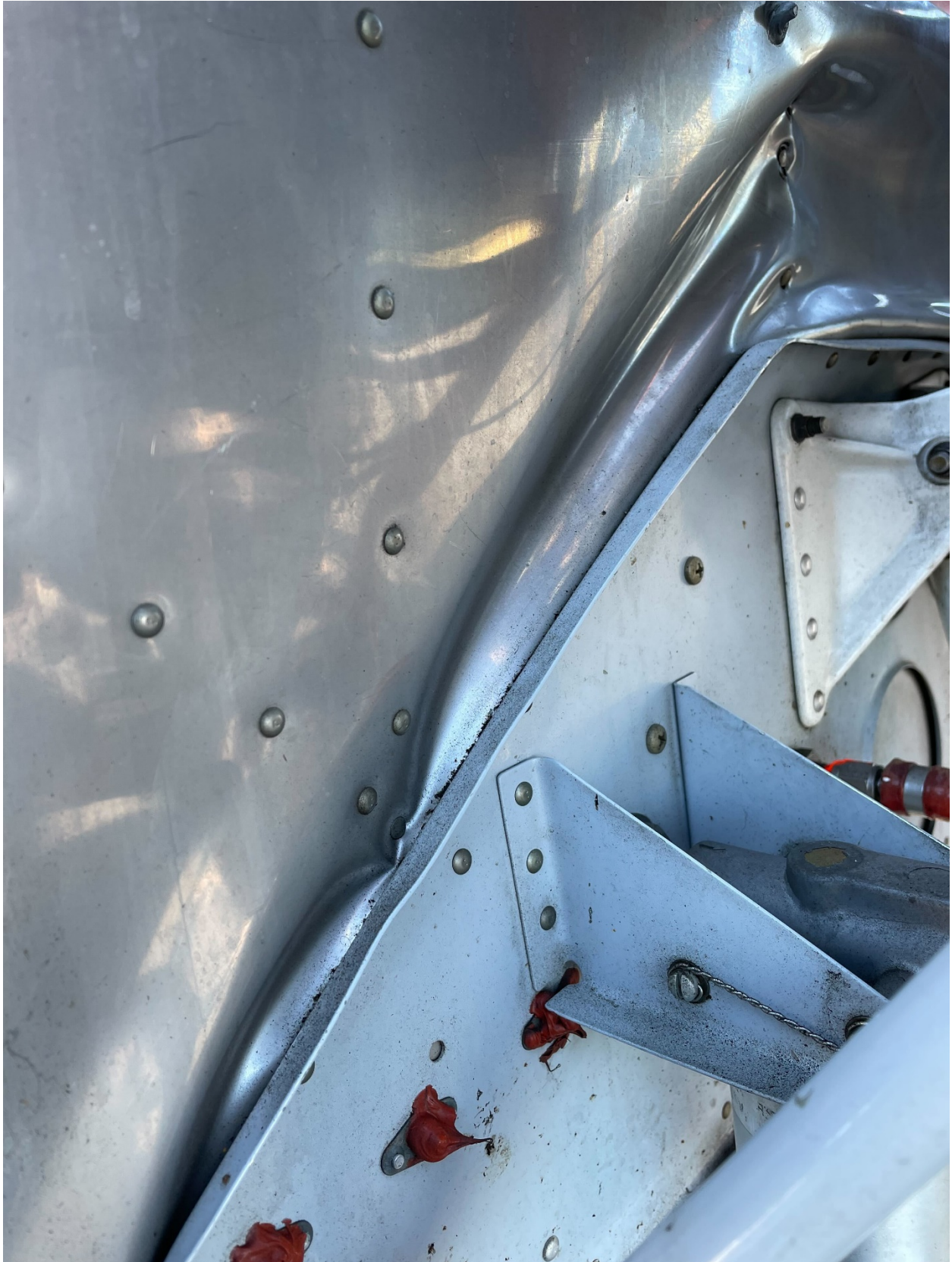
Photograph 3 – Accident airplane – Firewall damage.
