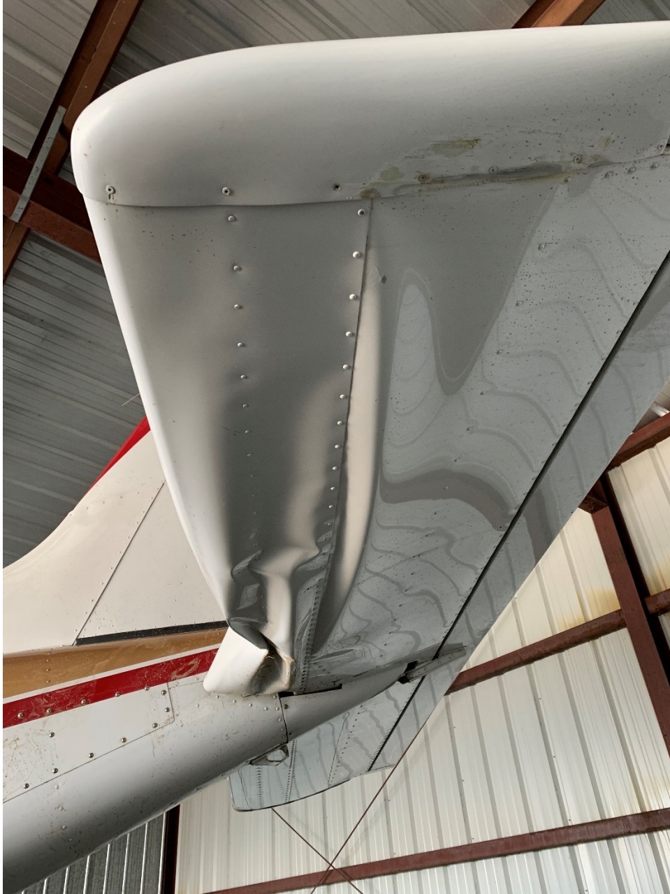
Photograph 4 4 – Accident airplane – left side horizontal stabilizer damage.
