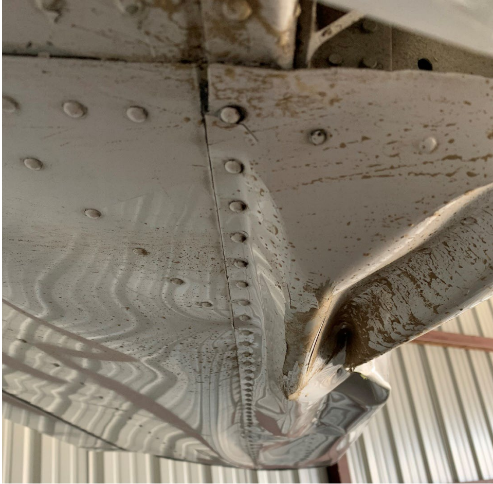
Photograph 5 5 – Accident airplane – left side horizontal stabilizer close up damage.
