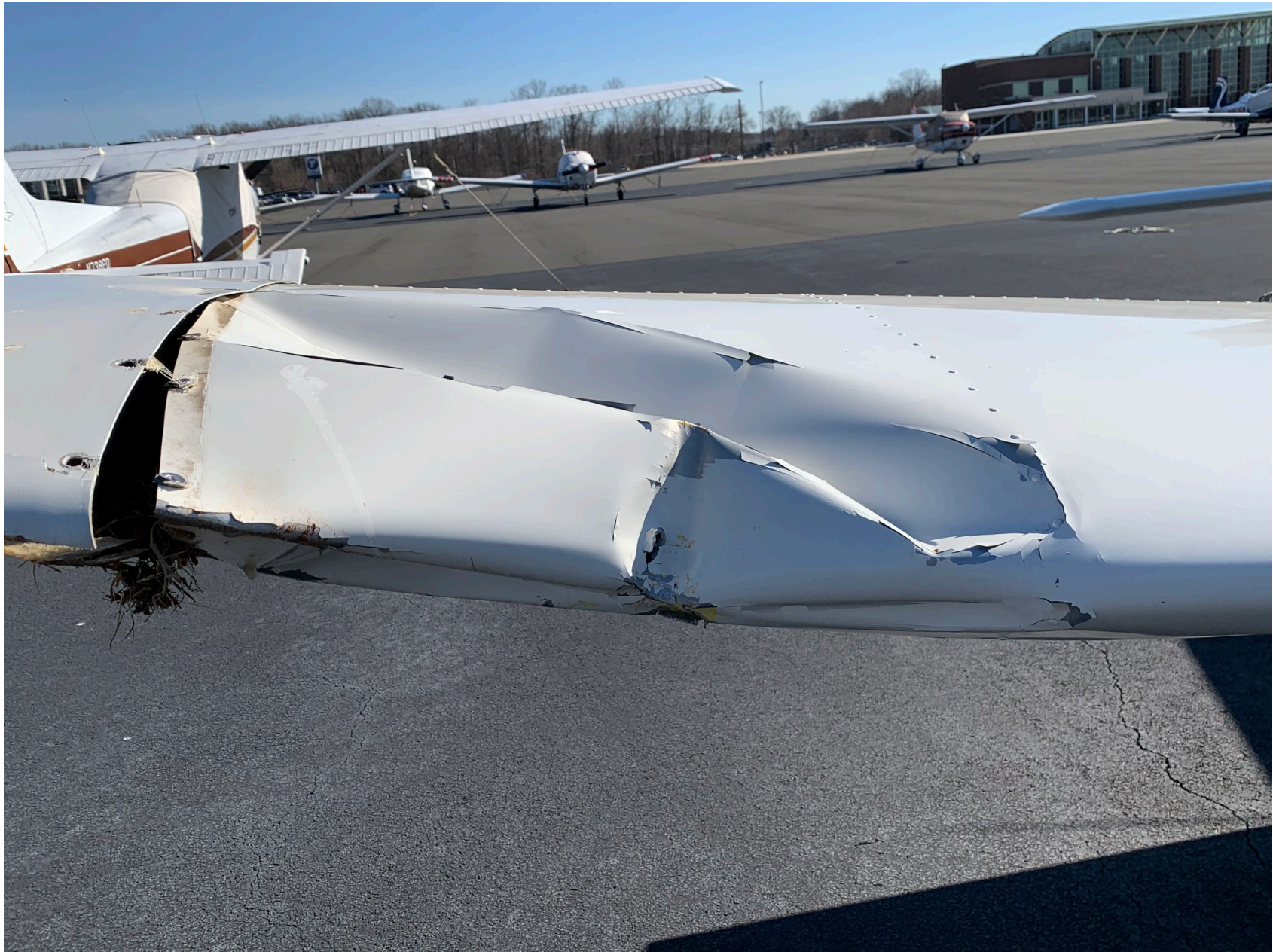
Photo 1 – FAA Digital Photograph. View of the damage to the Outer section of the Right Wing.
