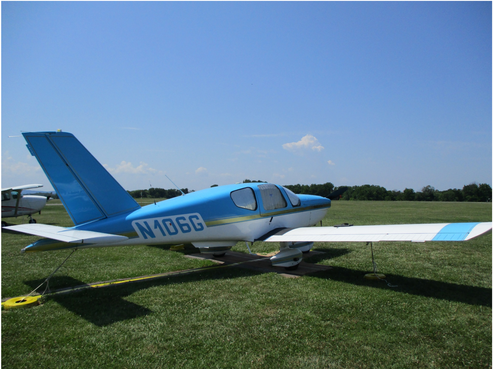
Photo 1 – right wing view, buckled wing
