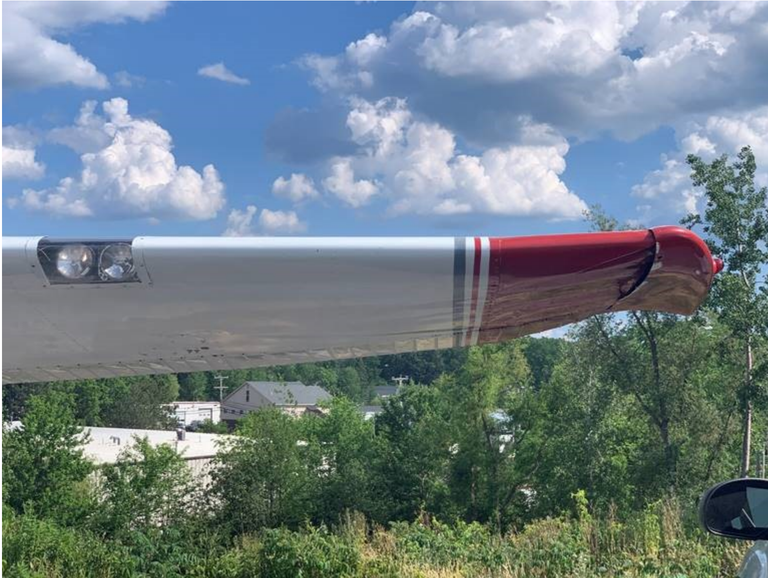
Photo 2 – Left wing tip, bent spar (Owner)
