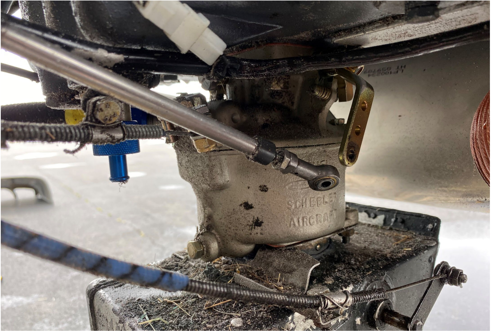
Photo 2 – throttle cable disconnected, bolt and nut missing (FAA)
