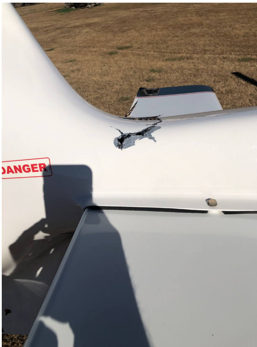
Photograph 2 - Substantial Damage to The Top of Tailboom (Courtesy of FAA)
