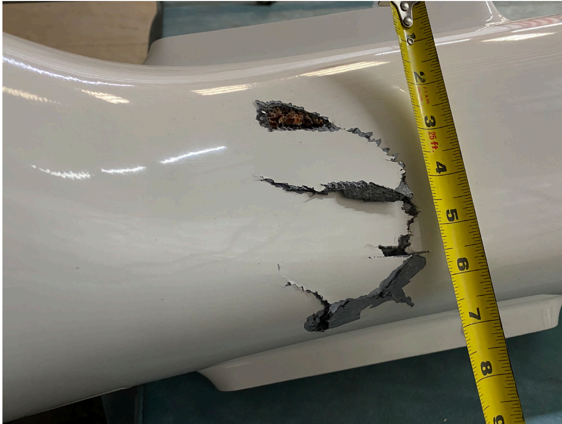
Photograph 3 - Closeup of Substantial Damage to Top of Tailboom (Courtesy of FAA)
