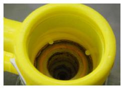
F Ensure that the purge point is inserted only to the center of the 1 1/4" end of the coupling.
