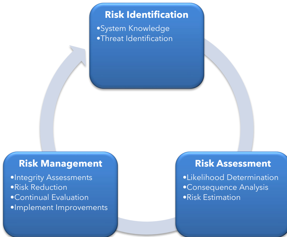
Figure 1. Integrity Management Flowchart
