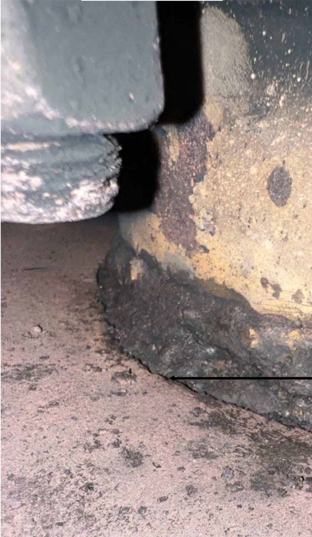
Photo #5 Cracked Muffler
