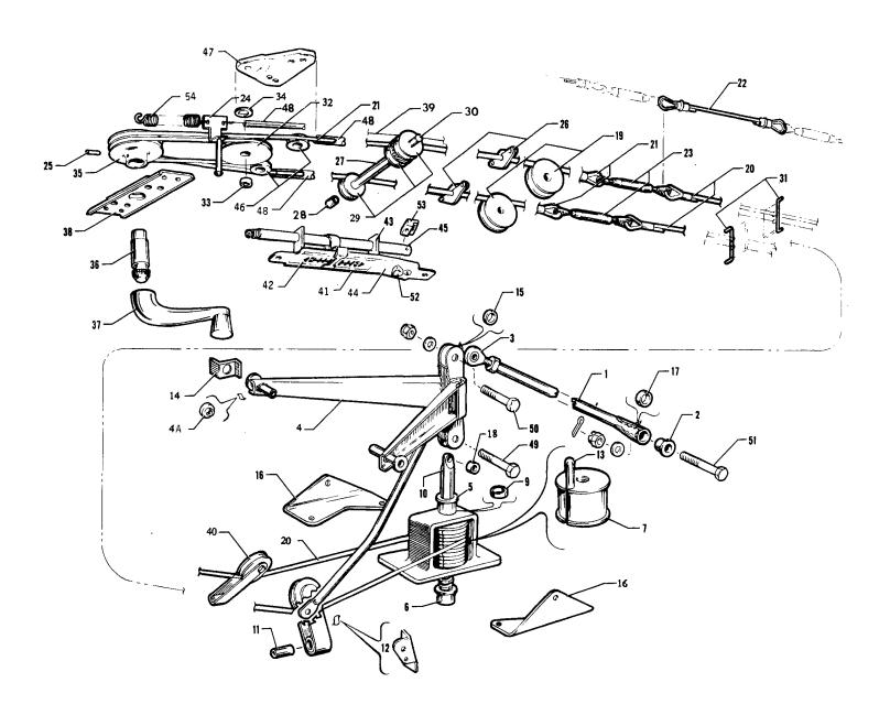
Figure 38. Stabilator Trim Mechanism Installation
