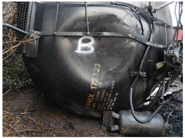
6(d) Dented B-end head.
