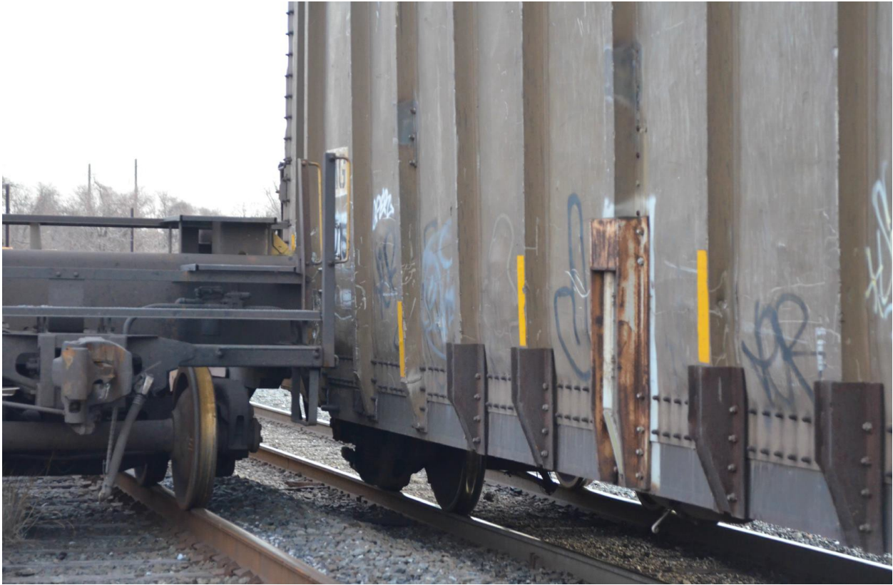
Figure 4- photo showing the high-side gondola passing the standing intermodal railcars. The intermodal railcars to the left of the picture are sitting on the Perryville track. Notice the limited clearance between the railcars.
