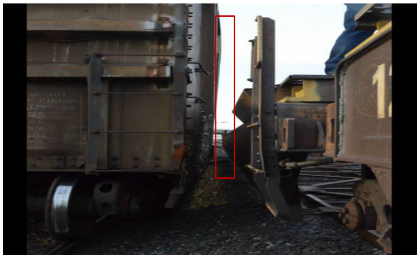
Figure 7- photo shows the limited clearance between the high-side gondola and the adjacent DTTX intermodal railcar.
