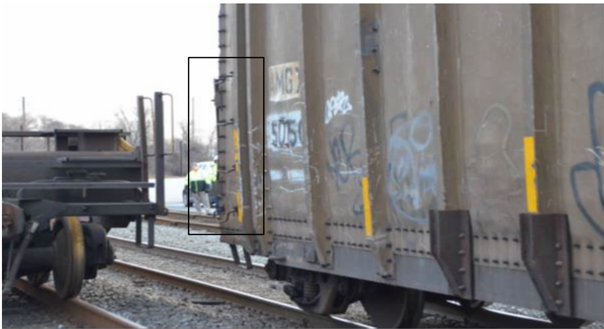
Figure 2- black rectangle indicates the location where the conductor was believed to be riding, while attempting to pass the standing DTTX intermodal cars on the adjacent track.
