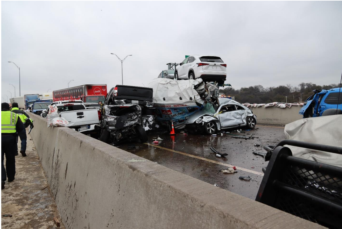
Highway Factors Photo 11 – View of damaged vehicles at the southern end of the I-35W southbound toll lanes crash scene standing on the left paved shoulder of the I-35W southbound general use lanes illustrating bags of coated salt on top of the concrete barrier used by first responders to treat ice on the roadway surface looking to the northeast (Source: Fort Worth Police Department. Photo taken on February 11, 2021, at approximately 8:04 a.m.)
