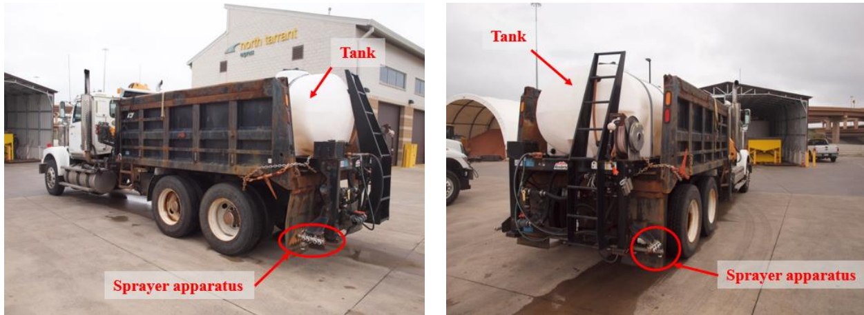
Figure 23 – NTEMP S3 truck and brine sprayer that applied the brine solution to the I-35W southbound toll lanes located at the NTEMP S3 maintenance facility (Source: photograph taken on April 29, 2021, by NTSB investigators).
