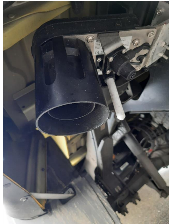
Figure 15 – Vaisala Mobile Detector MD30 mounted beneath the front and rear bumpers on MassDOT vehicles (Source: MassDOT).
