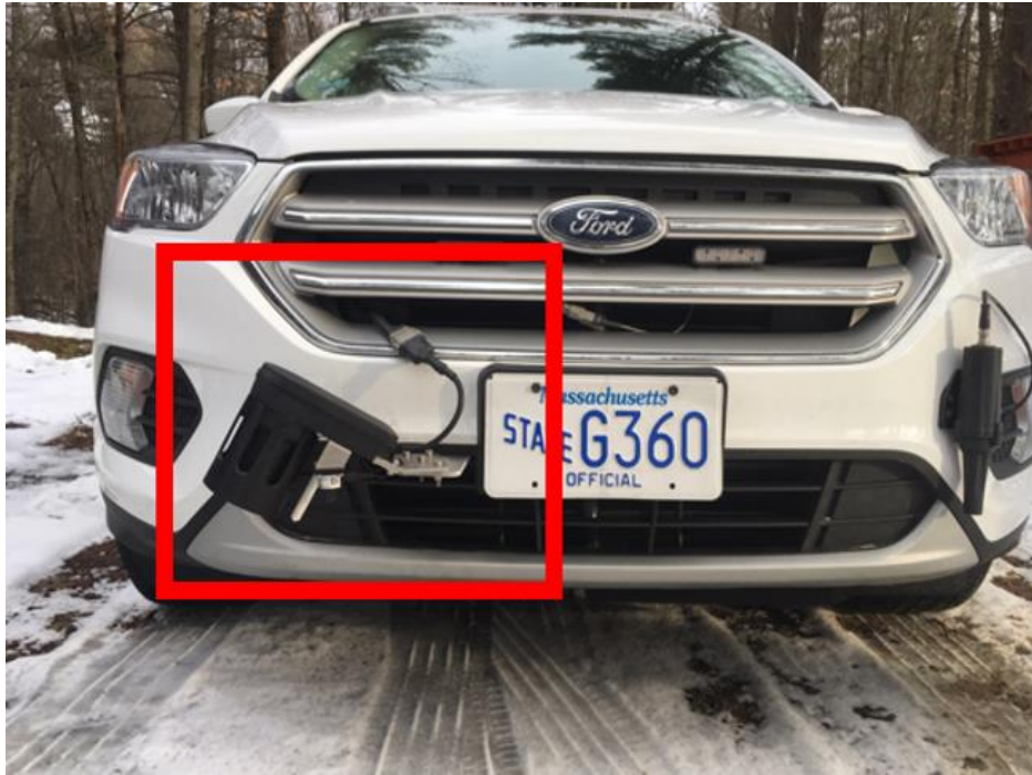
Figure 14 – Vaisala Mobile Detector MD30 mounted on the front bumper of a MassDOT vehicle (Source: MassDOT).
