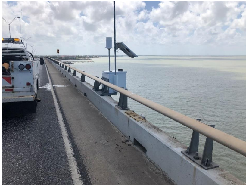
Figure 11 – Environmental Sensor Station (ESS) used in the Pharr District on SH100 (Queen Isabella Causeway) connecting Port Isabel with South Padre Island looking in the westbound direction (Source: TxDOT).
