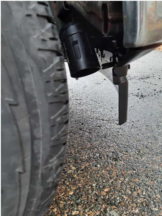
Figure 15 – Vaisala Mobile Detector MD30 mounted beneath the front and rear bumpers on MassDOT vehicles (Source: MassDOT).
