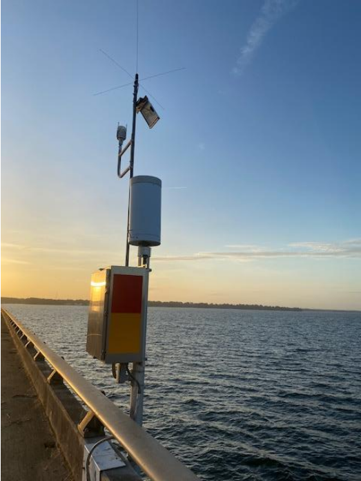
Figure 10 – Environmental Sensor Station (ESS) used in the Houston District on FM1097 (Rotary Friendship Bridge) over Lake Conroe looking in the eastbound direction (Source: TxDOT).
