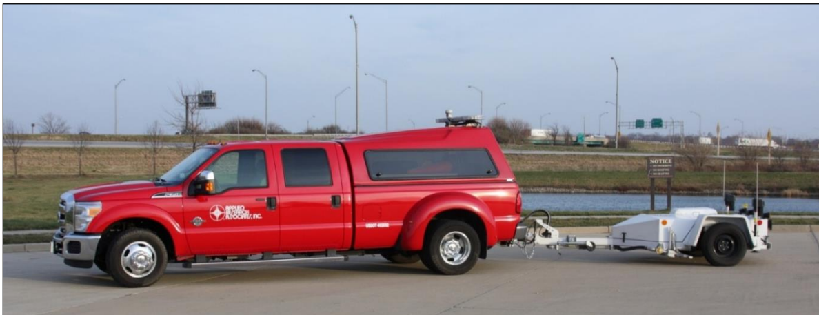
Figure 10 - Pavement Skid Friction Testing Equipment
