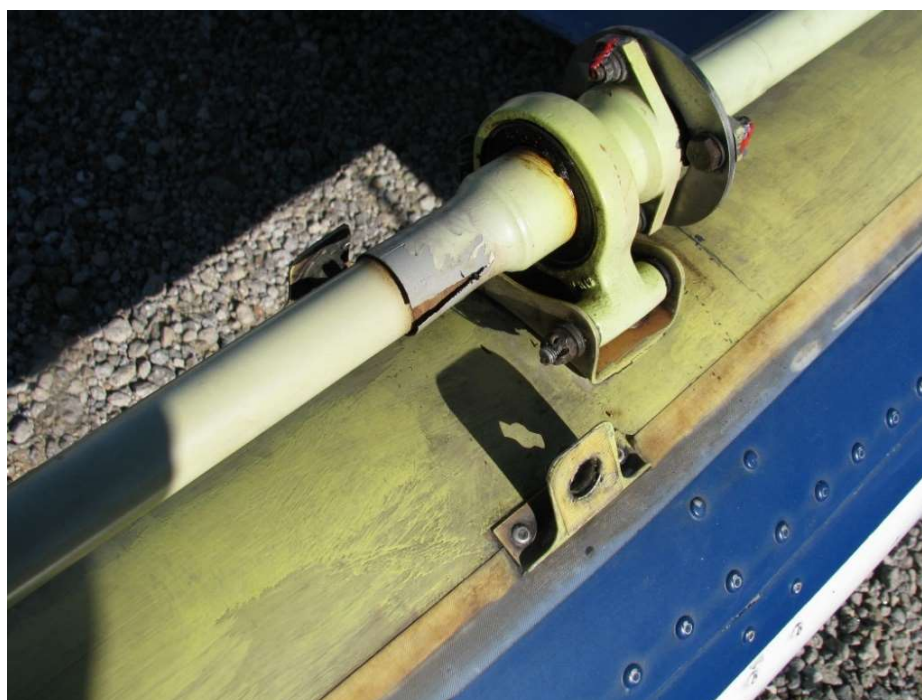
Figure 2. The separated splined adapter at the forward end of the No. 4 segmented tail rotor drive shaft. (Image courtesy of Bell)
