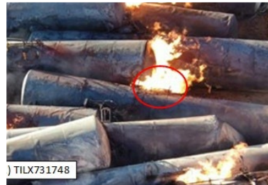
7(e). Flame from manway and top fittings housing.
