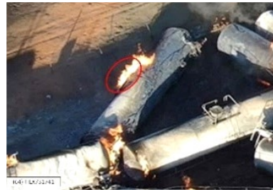
17(e). Flame in area of top fittings housing and manway.
