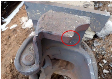
8(e). B-end coupler upper shelf sharp radius witness mark.
