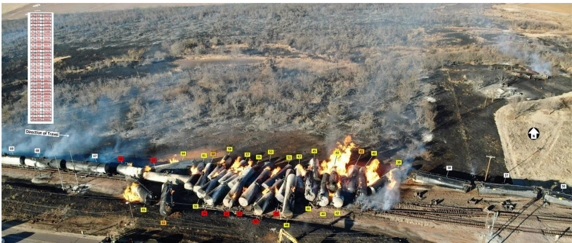
Figure 21. Breached tank cars in-situ with orientation marks.
