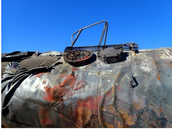
Figure 13. Missing top fittings protective housing with all top fittings sheared from flange. TILX 731462. Courtesy Trinity Industries Leasing, Inc., January 9, 2022.
