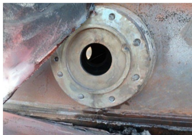
1(b) Full BOV assembly sheared away from the saddle.
