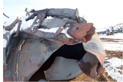
5(c). Fractured/torn B-end head with outward deformation of material.
