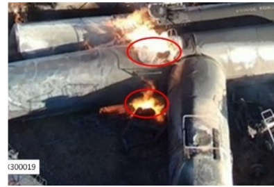
14(c). Flames at top fittings protective housing, manway, and bottom outlet valve areas.
