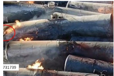
8(f). Flame at A-end head/shell tear.
