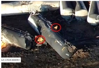
15(a). Flames at bottom outlet valve and manway.
