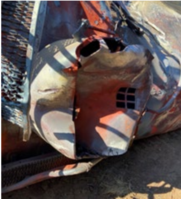
Figure 14. Mechanically damaged top fittings protective housing. CRDX 300133. Courtesy Federal Railroad Administration, January 11, 2022.
