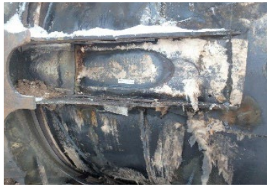
17(d). A-end inboard stub sill tail pieces. The measured A-7 fillet weld was adjacent to the white photo-tape.
