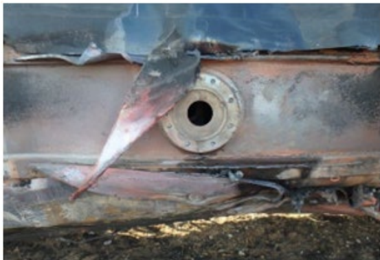
Figure 8. Skid structure missing/sheared away along with full BOV assembly and ball valve. Angular flap of center skid remains. TILX 731680. January 27, 2021.
