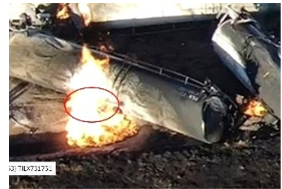
16(i). Flame from top fittings and manway area. The breached A-end head is to the right in this photograph with no flames visible in that area.
