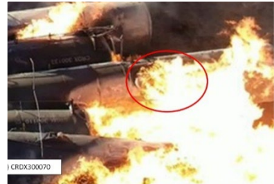
3(c) Flames from top fitting protective housing and manway area.
