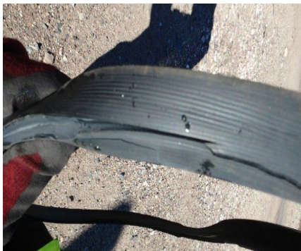
Figure 3. Nitrile rubber Buna-N manway gasket removed from TILX 731757 (#72) for lab analysis (Control# HMD22LR001-HAZ-004). January 28, 2022.
