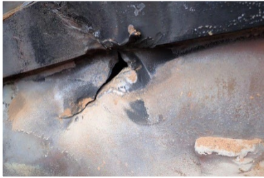
6(a). Tank puncture A-end bottom center, 2 ft. beyond BOV skid structure.
