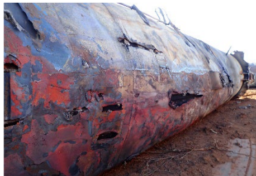
2(a) Heavy thermal and mechanical jacket damage. Missing bottom outlet valve and saddle, and collapsed skid protection structure.
