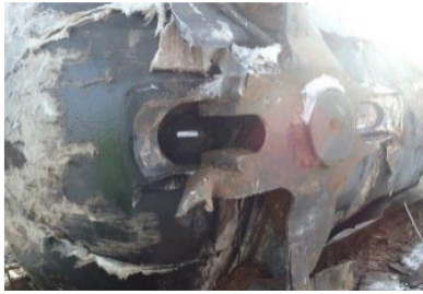
17(a). The A-end stub sill was fractured from the head brace with a piece of its broken web bent to the right.
