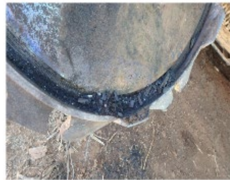
Figure 4. Thermally damaged manway elastomeric Buna-N gasket reduced to carbon, TILX 731758 (#65). Removed for lab analysis (Control#HMD22LR001-HAZ-006). January 28, 2022.
