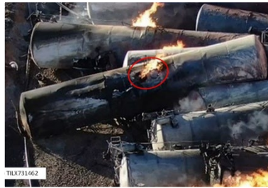
4(d). Flames from top fittings area.
