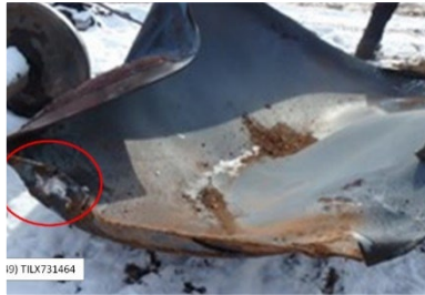
5(b). B-end head shield, impact mark (circled).
