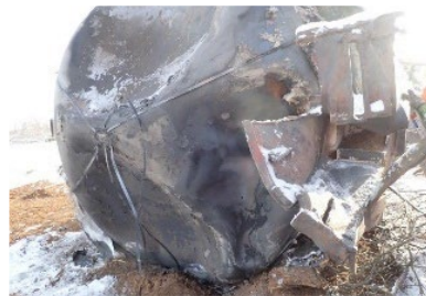
16(e). Stub sill web damage.
