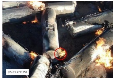
18(e). Flame indicates undocumented breaching damage at A-end head/shell interface, about 2:00.
