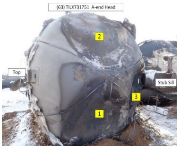
Figure 17. A-end head identifying three localized impacts, TILX 731751. January 27, 2022.
