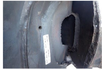
16(c). Fractured A-end head beneath fractured and separated head pad.
