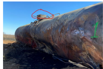
1(c) Protective housing cover torn off and crushed.
