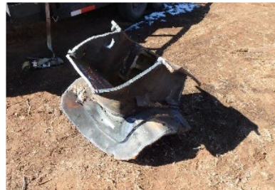
16(h). Evidence no. HMD22LR001-HAZ-002, stub sill/head pad/tank section.
