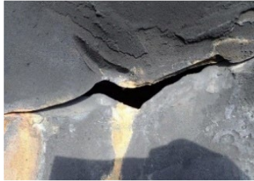
19(b). B-end head puncture and gouge.
