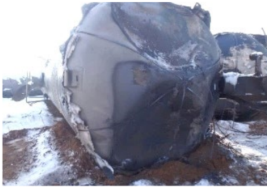
16(a). A-end head after head shield and jacket removal.
