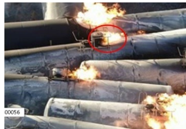
14(e). Flames from top fittings protective housing.
