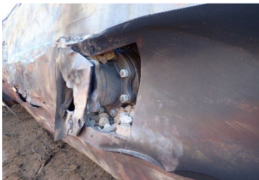
2(b) Bottom outlet valve sheared off with ball intact.
