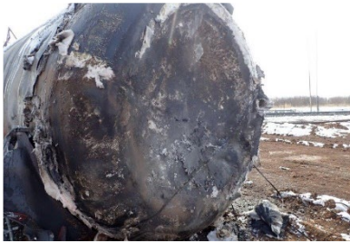
14(a). Rounded dent to A-end head as seen after head shield removal.
