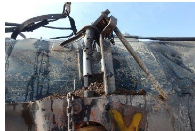
13(c). Bent and separated BOV operating handle extension.
