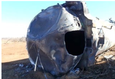
16(g). A-end head after stub sill/head pad/tank section was removed for laboratory examination.
