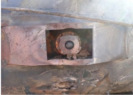
Figure 6. BOV nozzle sheared off. Valve body remained intact and closed at skid shear plane. TILX 731782. January 11, 2022. Courtesy Trinity Industries Leasing, Inc.
