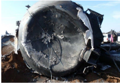
7(a). B-end head, rounded dent, fractured stub sill.
