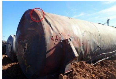
18(d). A-end breach location as indicated by flames in aerial imagery.
