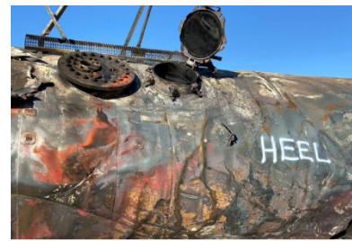
4(c). Thermally damaged manway and sheared shop fittings.
