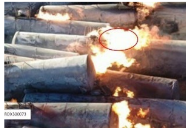
11(e). Flames in manway area.
