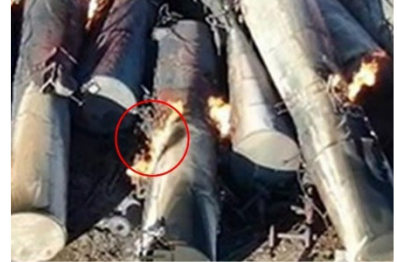
6(c). Flame in area of tank puncture, bottom center A-end side of BOV.
