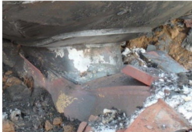
2.1(b) A-end head brace and pad with fractured head brace-to-stub sill weld.
