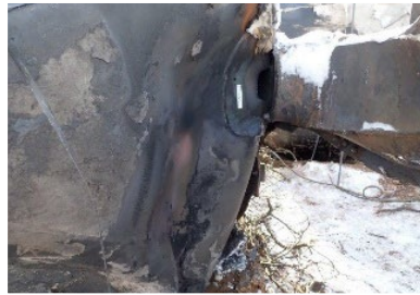
16(b). A-end stub sill and head damage.
