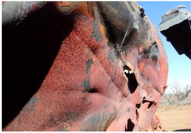
2.1(a) Buckled A-end stub sill. Head brace and pad.
