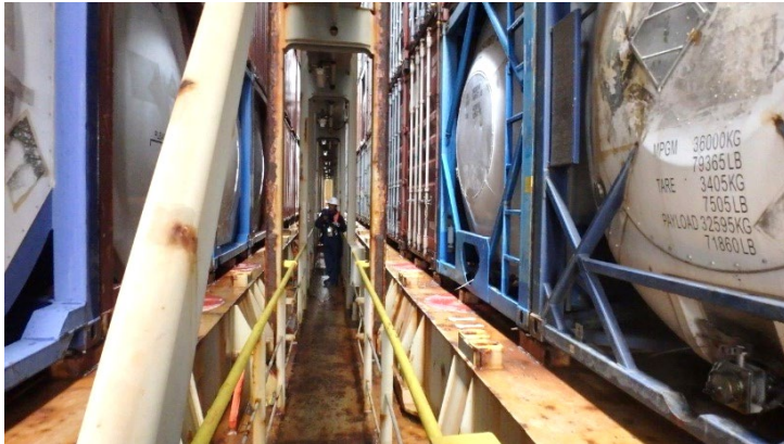
Figure 22. Iso-tanks stationed in Bay 15 (right) and Bay 17(left). No evidence of material releases were observed. March 28, 2024.
