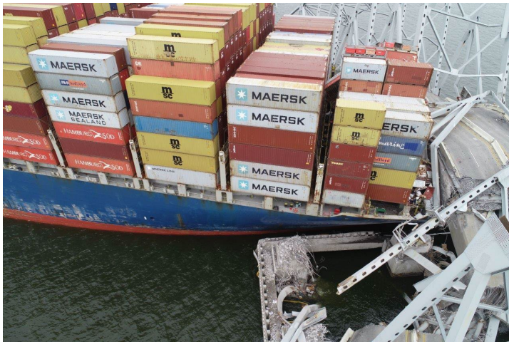
Figure 3. ISO 20 and 40-foot shipping containers stowed in Dali forward above deck cargo bays and fallen bridge debris on the bow, March 28, 2024.
