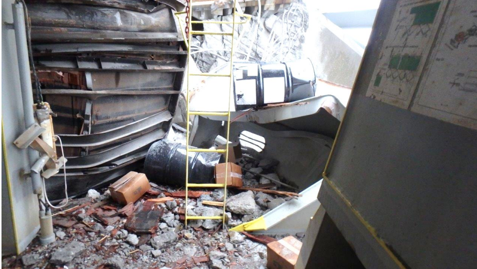
Figure 20. 55-gallon drums of Weston 705T that had come to rest on the main deck. The bottom surface of the damaged cargo container is visible on the left side of the photograph. March 28, 2024.
