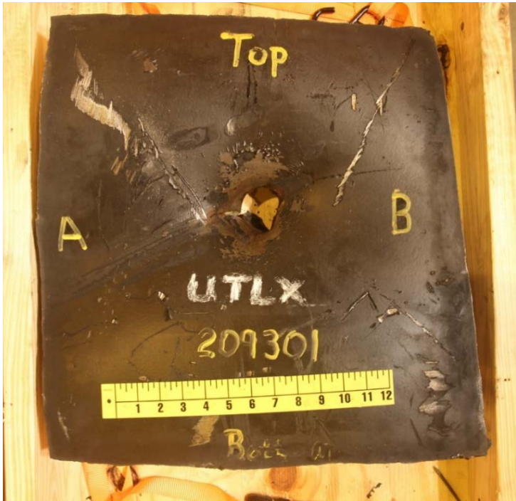
Figure 1. UTLX 209301 shell coupon with puncture, left side Ring 2.
