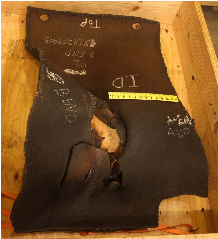
Figure 4. UTLX 209403 breached B-L shell plate interior surface.
