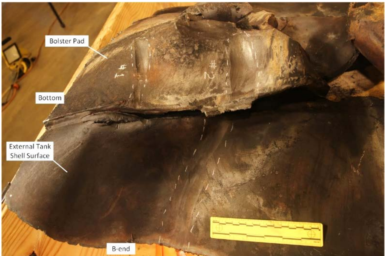
Figure 10. UTLX 209403 tank shell coupon from B-L bolster region showing outlined extent of wheel bum marks at locations #1 and #2.
