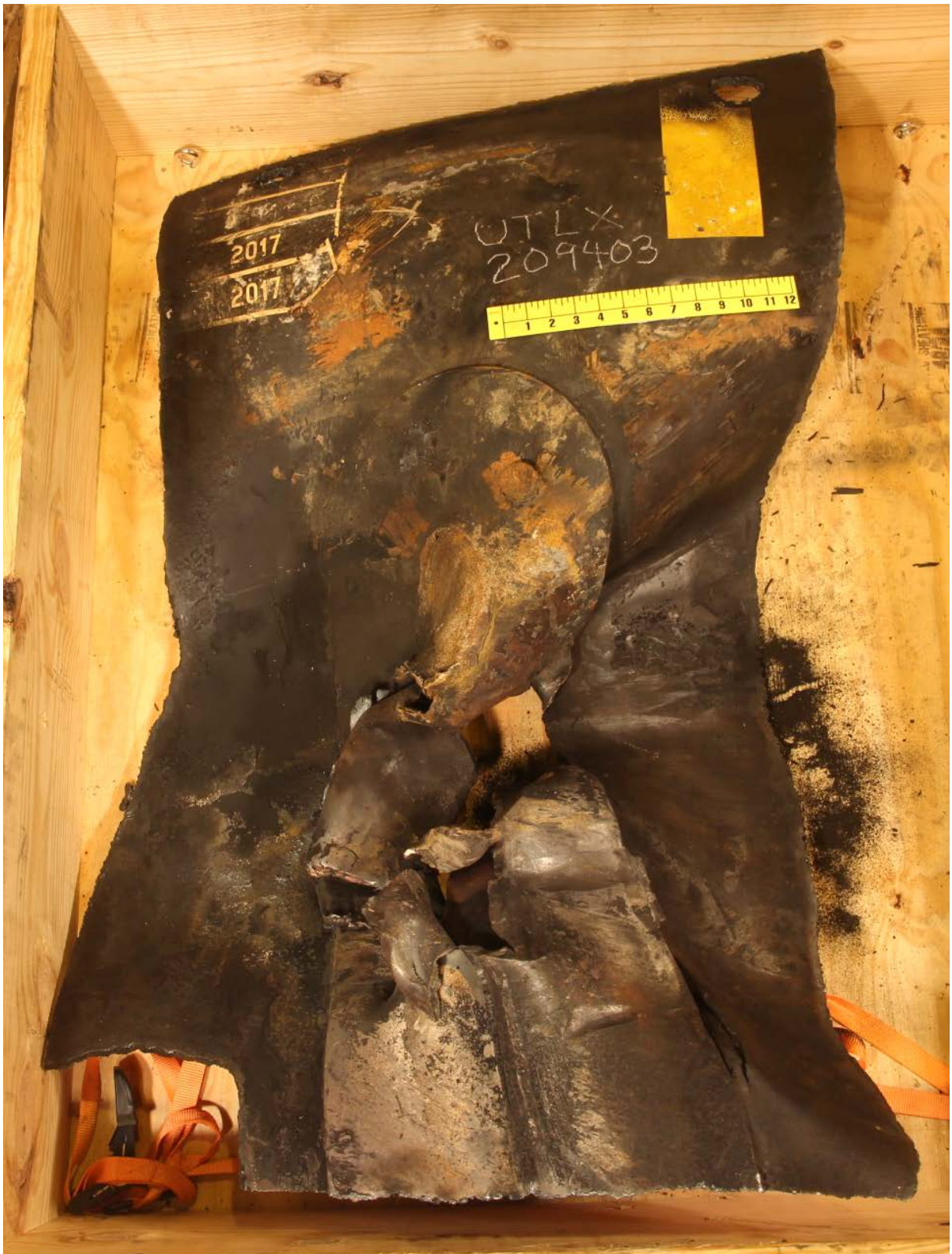
Figure 5. UTLX209403 breached shell plate with B-L body bolster pad, exterior surface.
