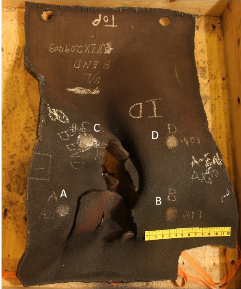
Figure 13. UTLX 209403 tank shell coupon B-L bolster region, ultrasonic thickness measurement locations A through D. Shiny circular areas are locations where corrosion was ground away before testing.
