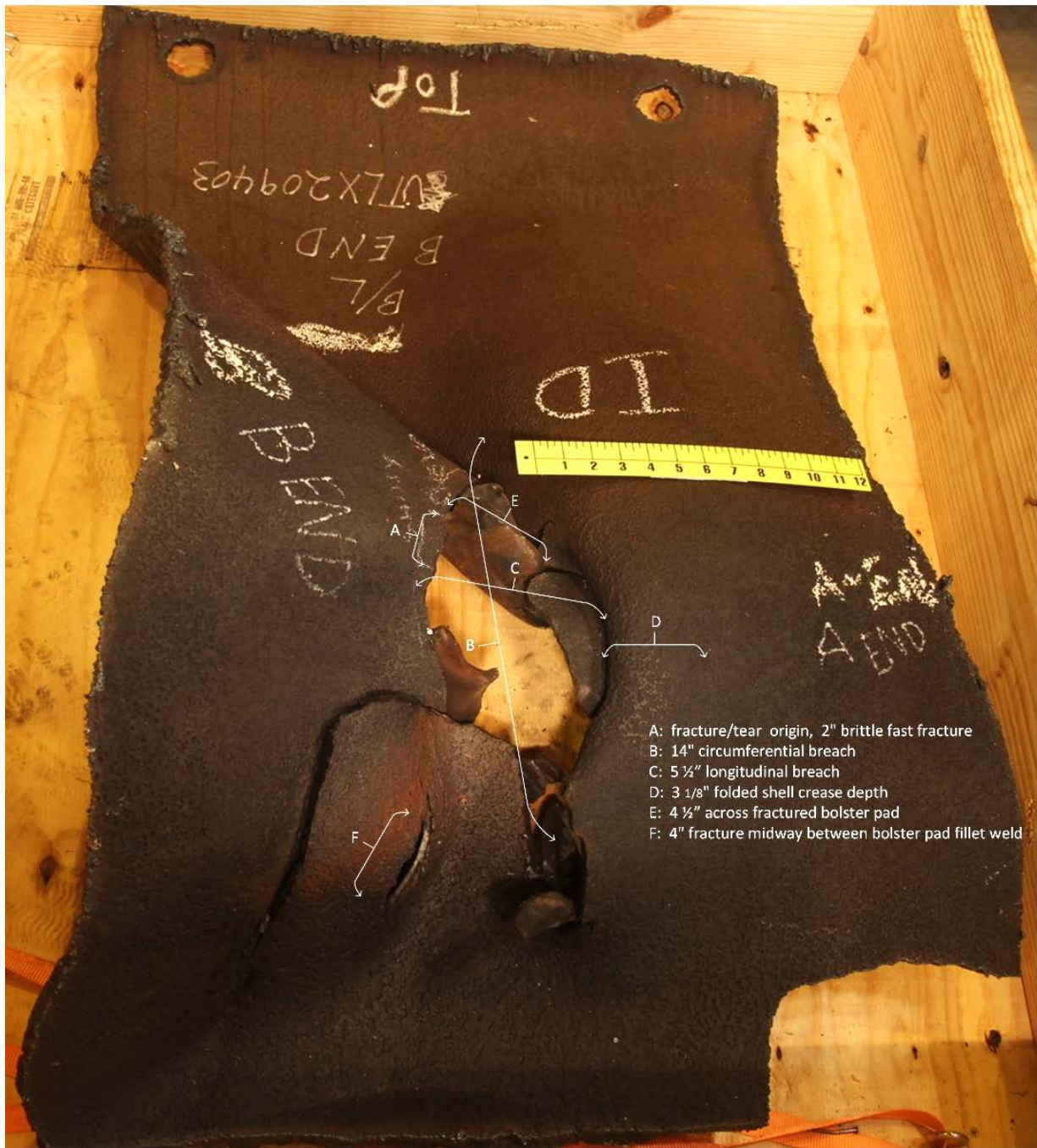
Figure 6. UTLX209403 tank coupon interior surface with noted measurements and fracture/tear features.
