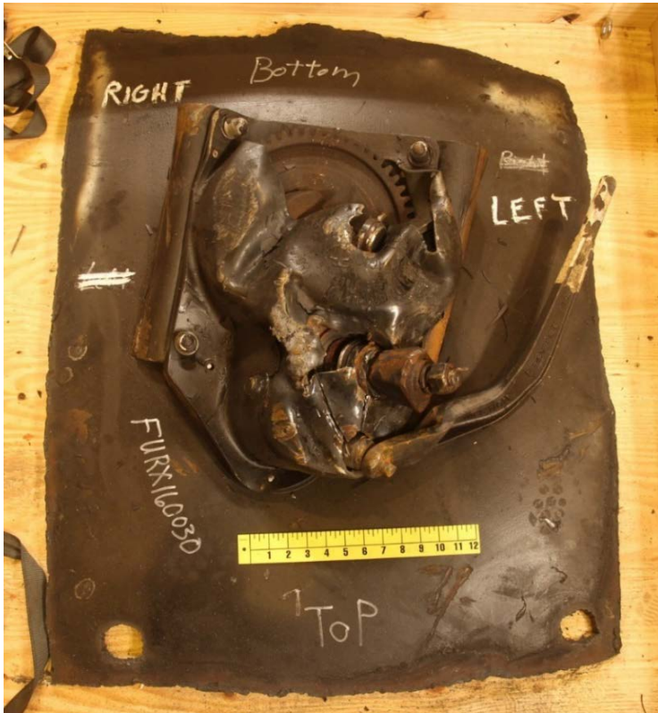
Figure 2. FURX160030 head shield coupon with hand brake assembly (missing hand wheel).
