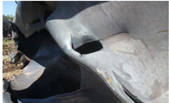
7(d) B-end head rectangular puncture and tear.
