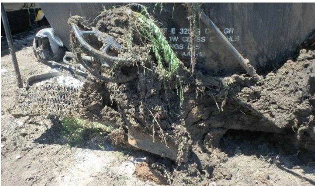
20(c) Fractured B-end stub sill and missing coupler.
