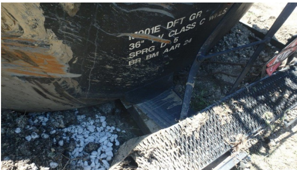
10(c) A-end head shield gouge about 6 o'clock.
