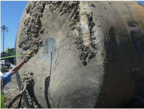
1(a) A-end head dent, 3' x4'
