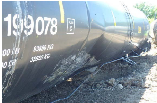
17(b) A-L dent, 5' x 8', depth was not measured.
