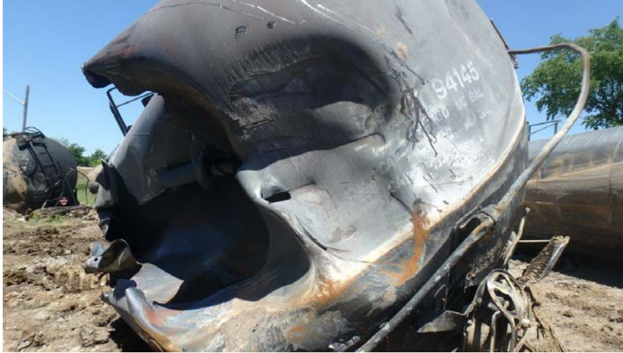
Figure 7. TCBX 194145, B-end head punctures and dents.
