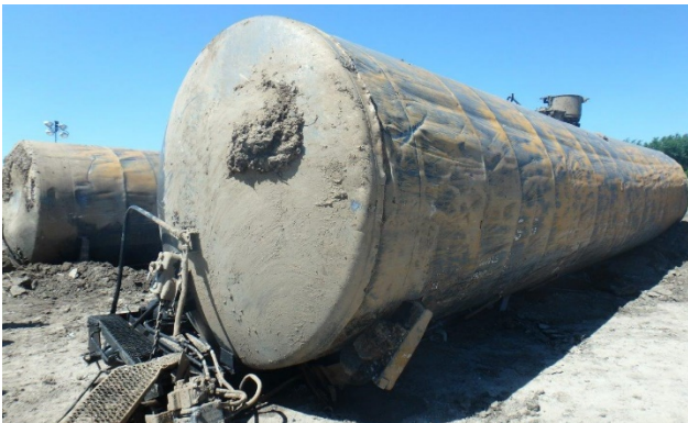
2(a) B-end head bent stub sill, right side shell with wrinkled jacket and scrapes.
