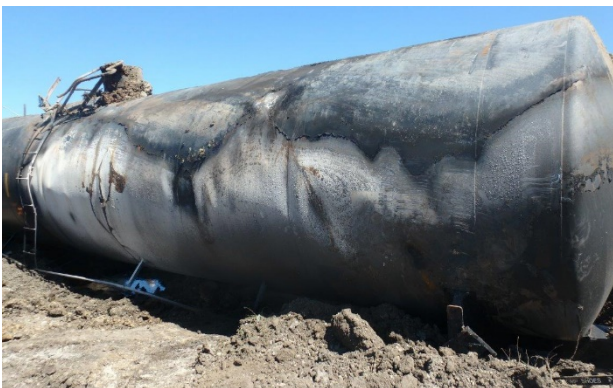
1(c) Thermal damage right side, center to A-end.
