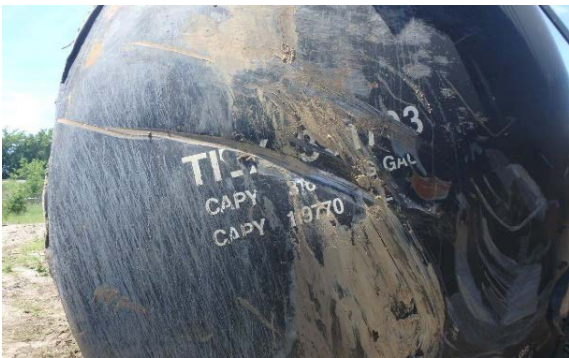
10(a) A-end head shield gouges about 10 o'clock.
