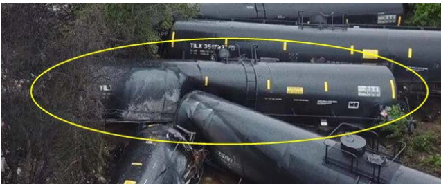
9(a) Resting position in the derailment scene with B-end of GATX 225797 in contact with the A-L shell.
