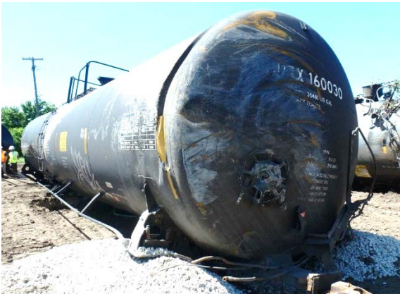
18(a) B-end head, crushed brake wheel and head shield gouges.
