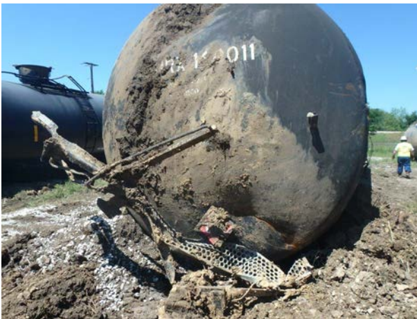
11(a) A-end head shield and gouge at 5-6 o’clock.
