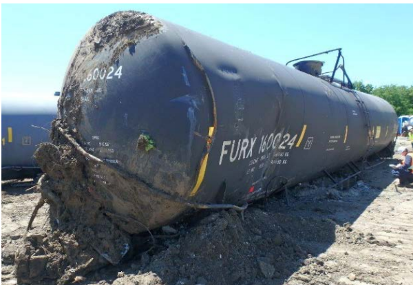
15(c) B-end head and B-R jacket dent, 5' x 5'.
