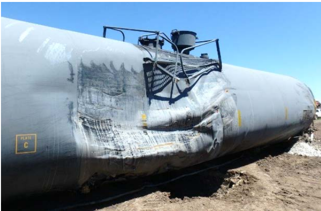
16(c) Left side overall impact damage.
