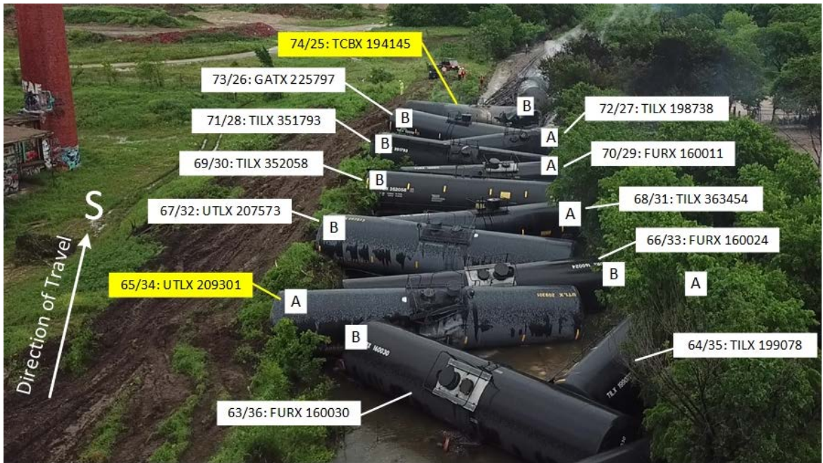
Figure 45. North end (rear) of the derailment. Leading ends are labeled.
