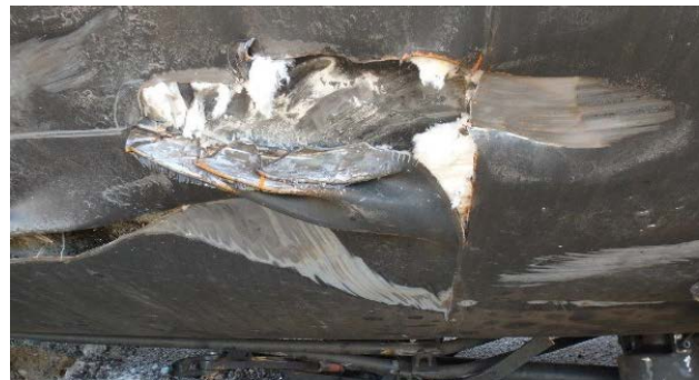
12(b) B-L jacket tear and non-breaching shell gouge.
