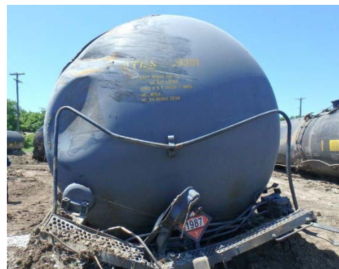
16(f) B-end head dents, 2' x 3' and 2' x 2'.
