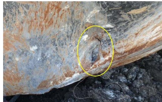
9(d) A-end head shield with 2" x 8" puncture.
