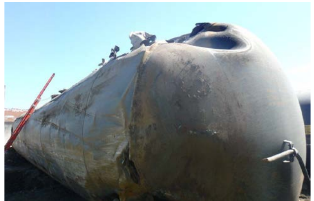
5(d) Deep B-end head dents at 11 – 12 o'clock.
