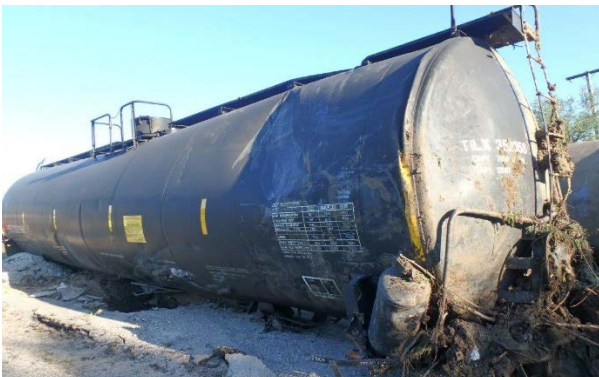
12(a) B-end head and B-L jacket dent.
