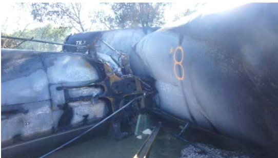
8(a) A-end stub sill of TILX 351873 wedged into the A-L shell as found in the derailment site.
