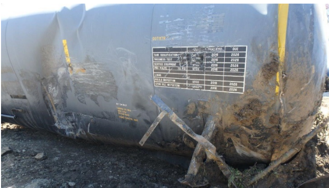
16(e) A-end head and A-R 4'x6' dent.
