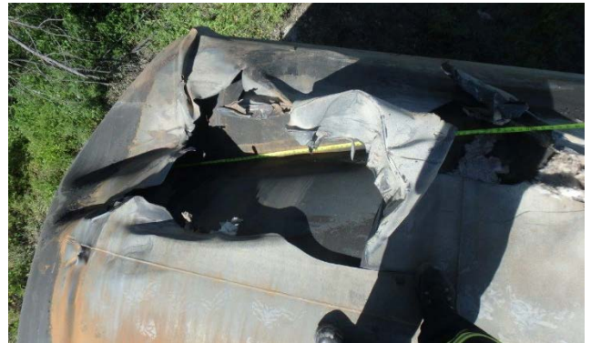
5(f) B-top jacket tear and dent 27" deep x 42" wide x 72 long.
