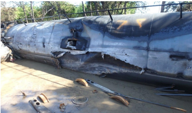
4(a) Tank bottom as found in the accident scene, showing thermal damage, with jacket tear and dent on B-L bottom.
