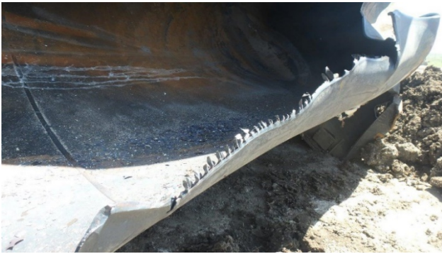
7(c) Bottom B-end shell breach with high-rate tearing fracture (sawtooth burrs) on bottom fracture surface.
