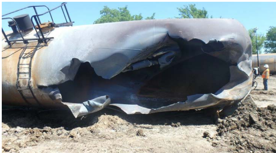
Figure 6. TCBX 194145, left side shell tear.
