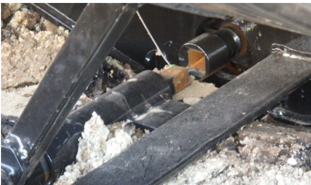
23(c) Disengaged BOV operating handle extension.
