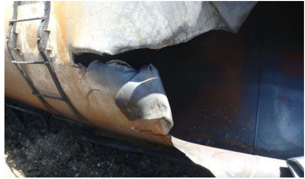
7(b) Inboard B-L shell tear detail.
