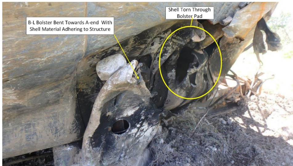
Figure 4. Shell tear, 6 x 13-inches, B-L bolster pad area
