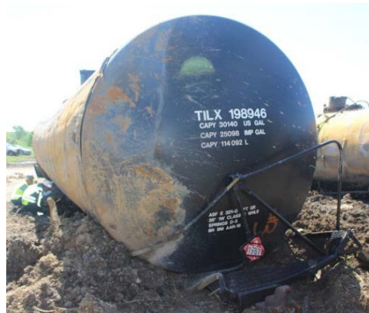
2(b) A-end head with dent at 10 o'clock.
