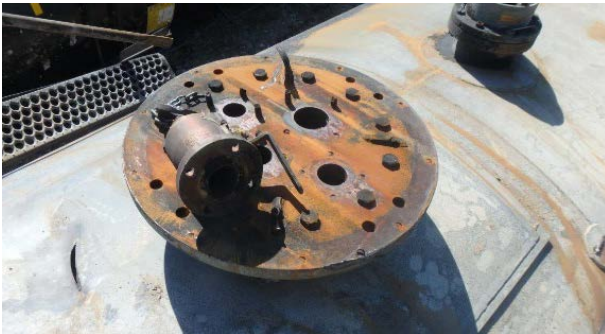
5(e) Top fittings flange with missing protective housing, liquid, vapor, and vacuum relief valves.
