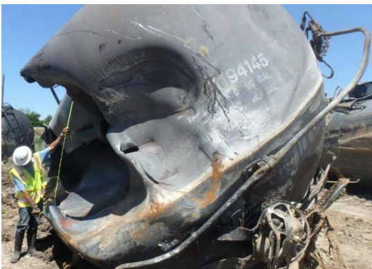
7(e) B-end head breaching damage.
