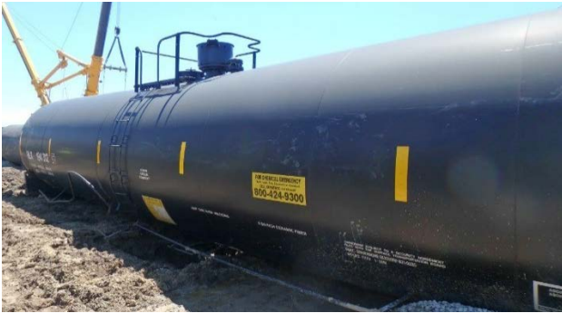
20(a) Left side showing no derailment damage.
