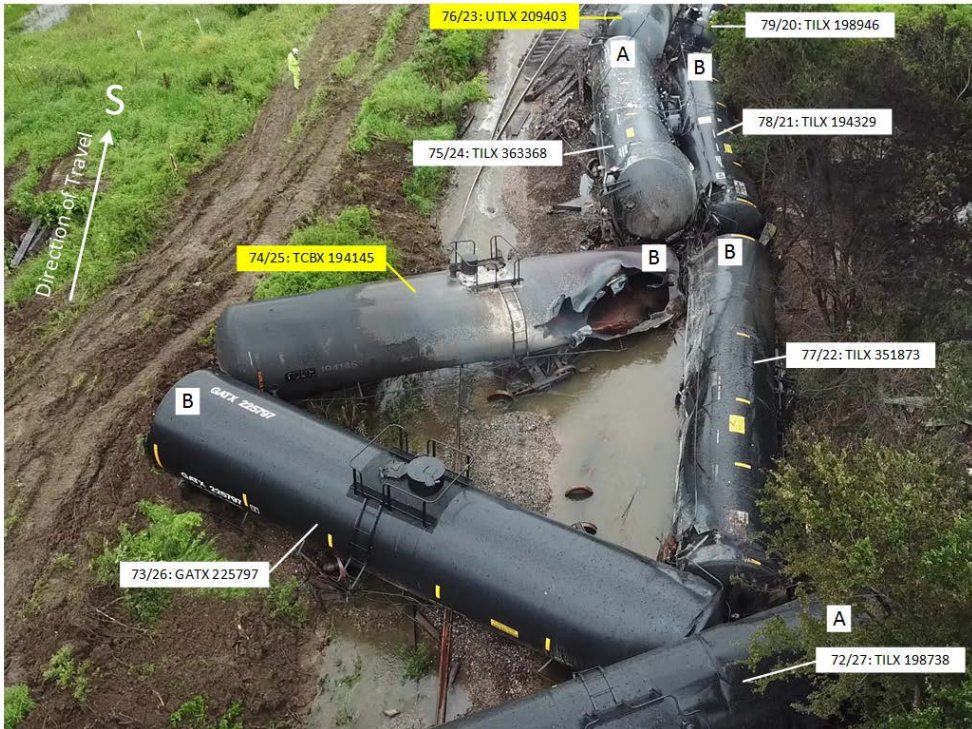
Figure 14. Middle of the derailment. Leading ends are labeled.
