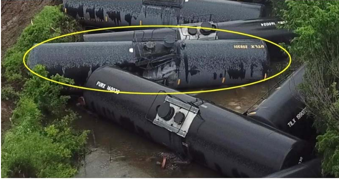
16(a) UTLX 209301 as found in the derailment scene, showing position of impacting car FURX 160030.
