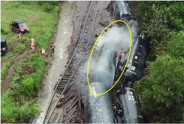
5(a) Car in the derailment scene on its left side with fire from top fittings impinging on adjacent car TILX 198946.
