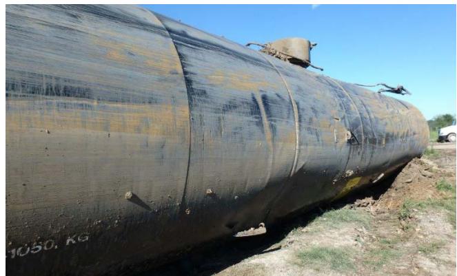
13(b) Right side, jacket wrinkles and scratches.
