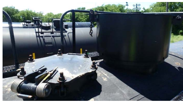
21(d) Transquip 6-bolt manway assembly under AAR service trial no. ST-470.
