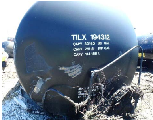
20(b) A-end head 2'x3' head shield dent at 8 o'clock.
