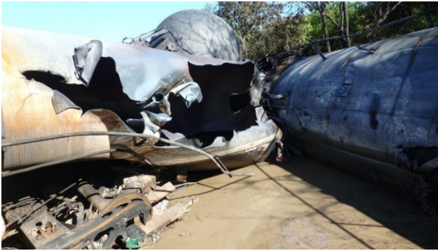
7(a) Car in the derailment scene showing the B-L irregular-shaped shell tear.
