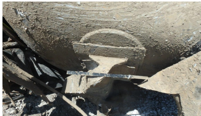
8(d) B-R bolster bent toward the B-end.
