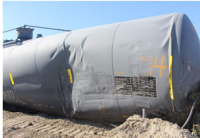
14(b) B-L dent/buckle, 5' x 8', adjacent gouge and scrape marks.
