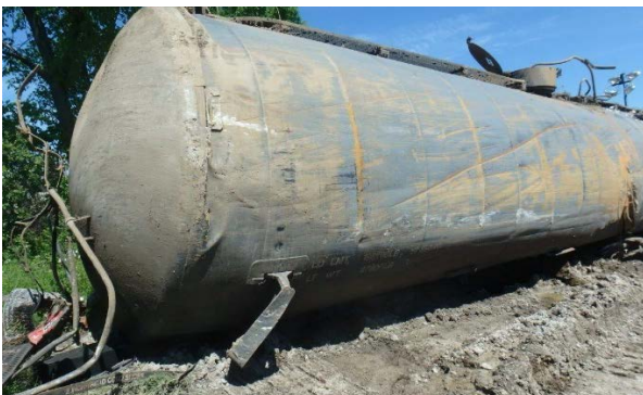
4(c) A-end and left side, bent A-L body bolster.
