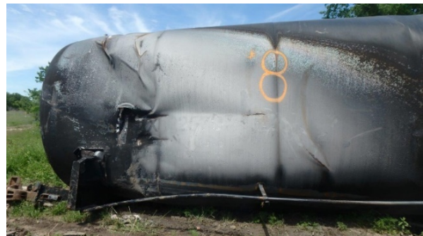
8(b) A-end impact location as seen in the staging area. Thermal damage to jacket paint.
