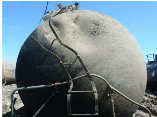
4(b) A-end head shield dents at 11 and 12 o'clock
