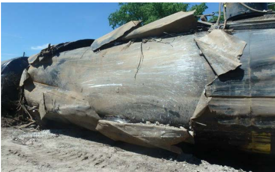
8(a) B-R side jacket tear and gouge. The gouge continued over jacket down the center left side.
