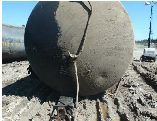
3(b) A-end head gouge at 5 o'clock.
