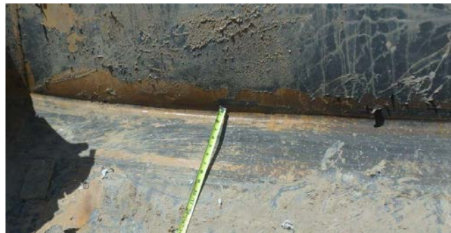
8(b) B-R gouge 116-inches in length, 2-inches wide.
