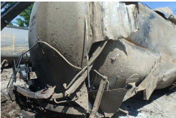
8(c) B-end head, with partially detached head shield.
