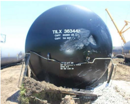
21(a) A-end head shield dent about 2 o'clock..
