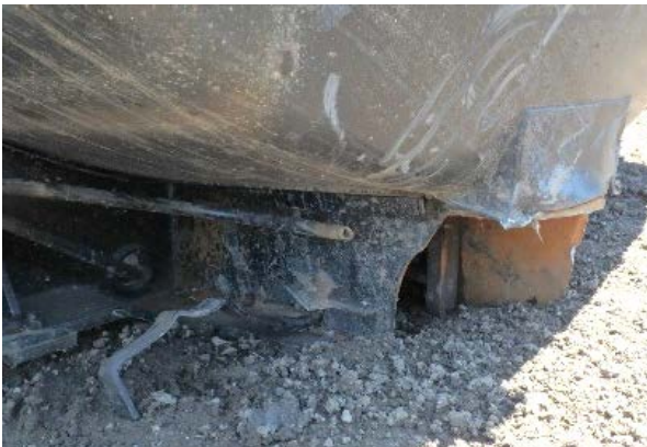
17(c) The B-end stub sill was fractured at the head brace.
