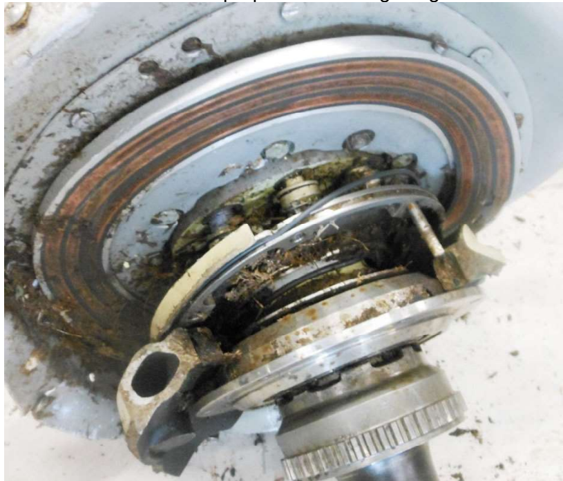
Photo #12 - Left propeller mounting flange area
