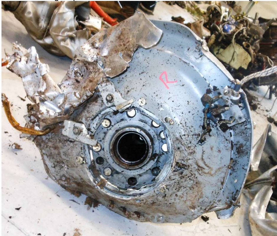
Photo #3 - Right spinner bulkhead and one start lock bracket fragments
