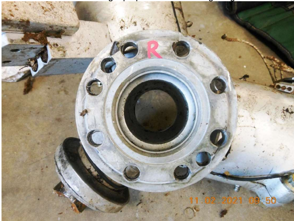
Photo #4 - Right propeller hub mounting flange
