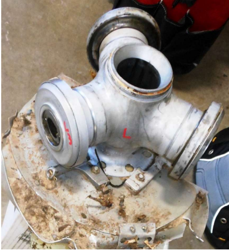
Photo #15 - Left propeller hub unit/spider
