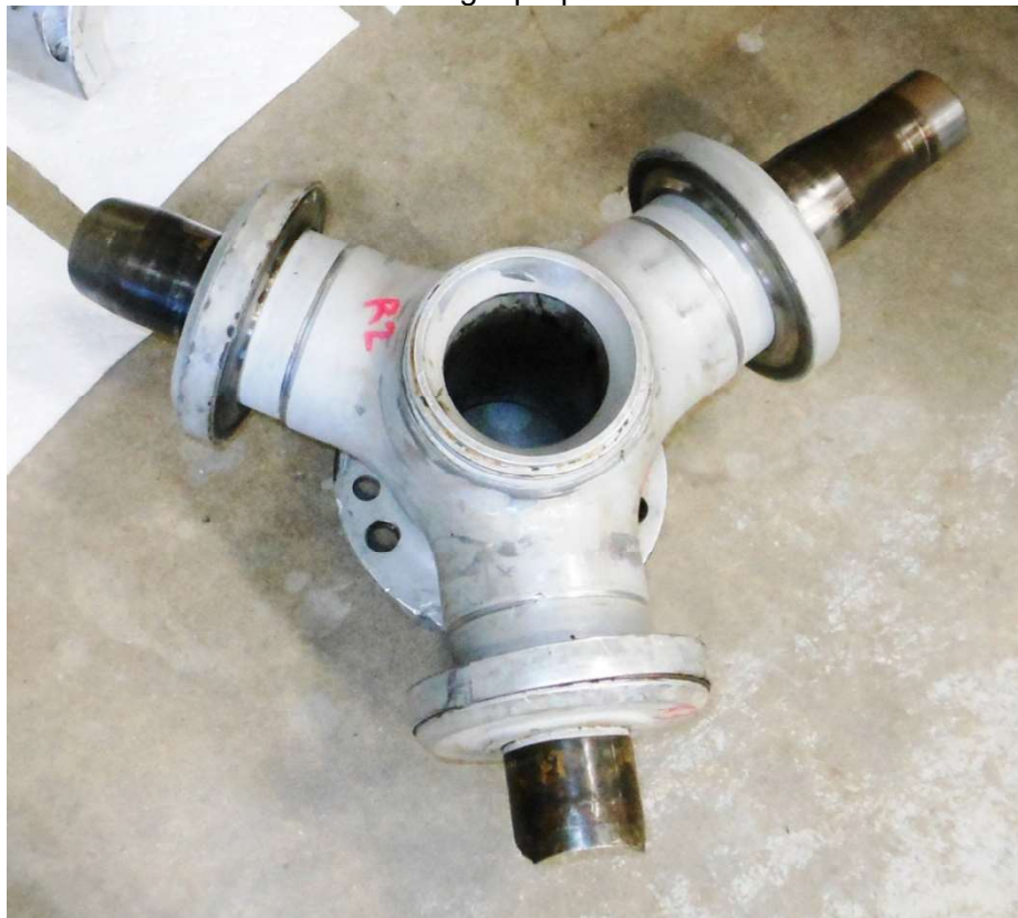
Photo #5 - Right propeller hub unit
