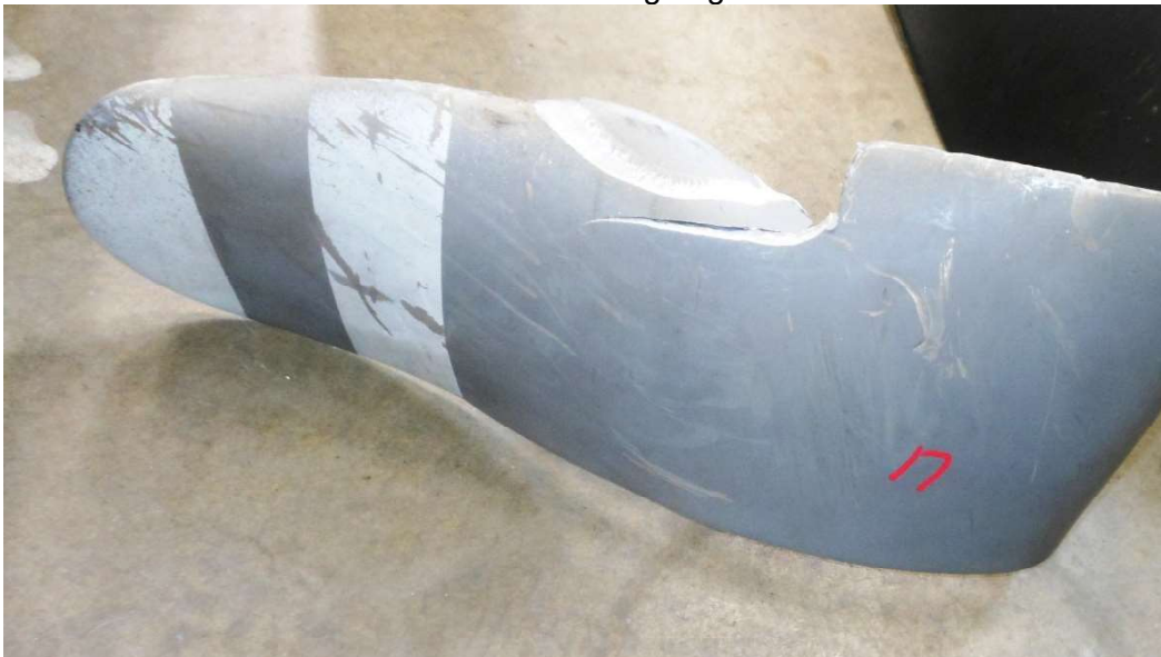
Photo #16 - L1 blade leading edge fracture/tear
