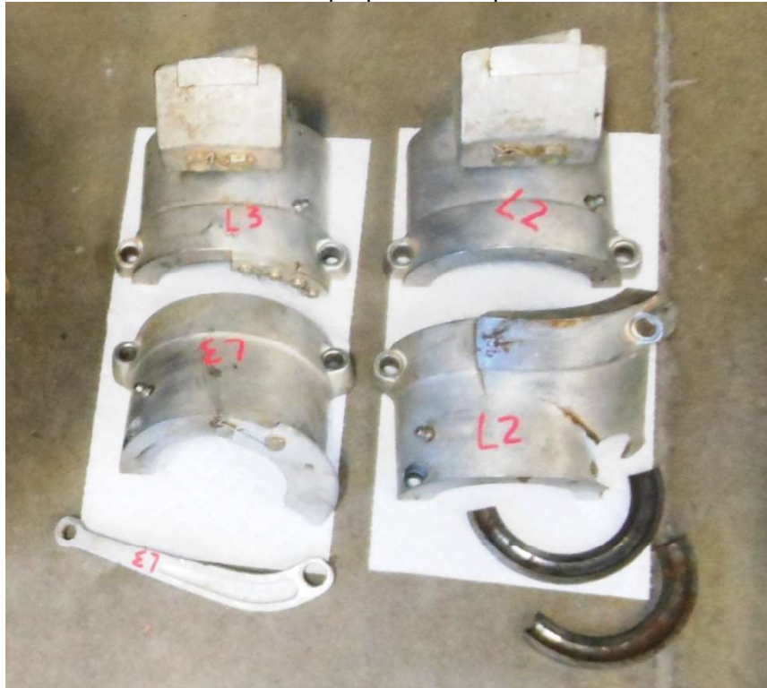
Photo #13 - Left propeller clamps recovered
