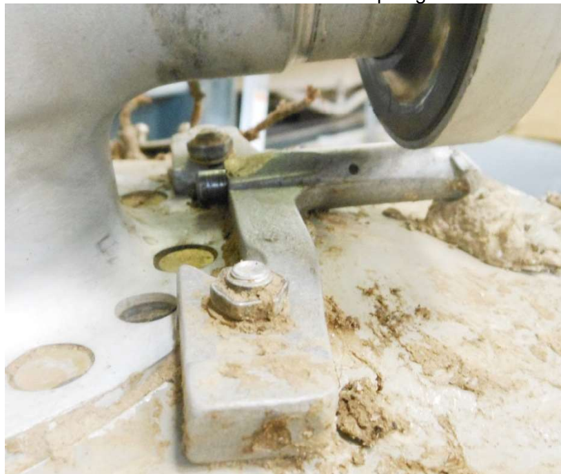
Photo #14 - L3 start lock bracket with plunger extended
