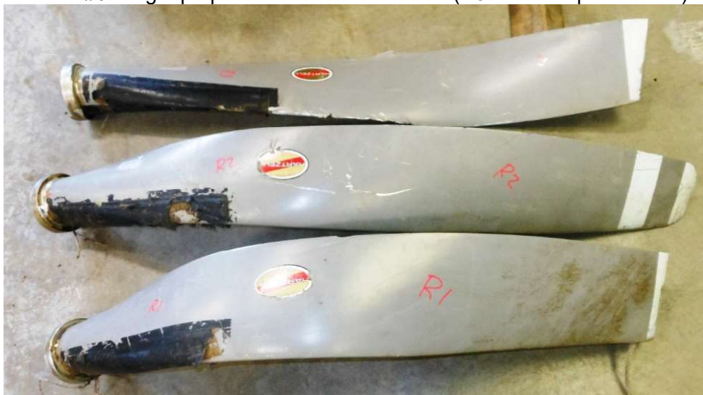
Photo #9 - Right propeller blades camber side (R3-R2-R1 top to bottom)
