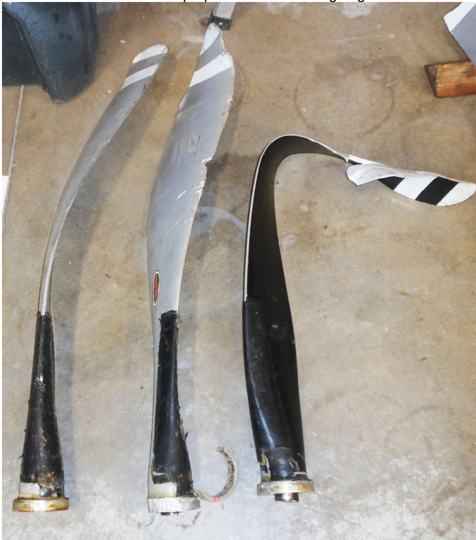
Photo #18 - Left propeller blades leading edge view
