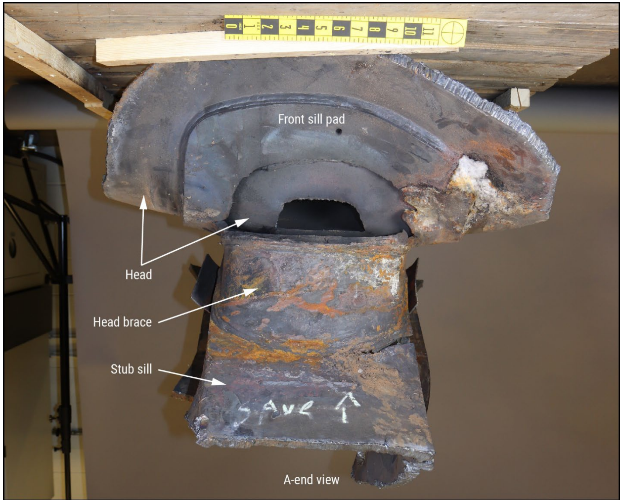
Figure 7. Head-on view of sectioned piece from tank car TILX731751.
