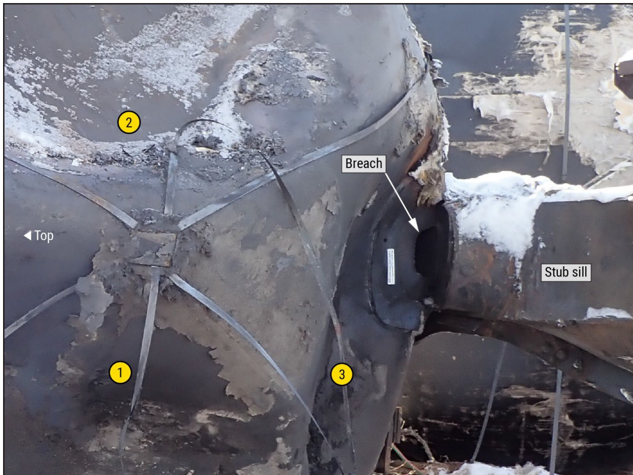
Figure 3. The A-end head of tank car TILX731751 postderailment and with the head shield removed for inspection, showing deformation from three impacts.
