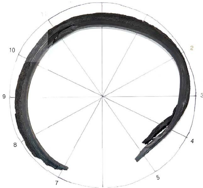
Figure 4. Manway cover gasket removed from tank car TILX731758.
