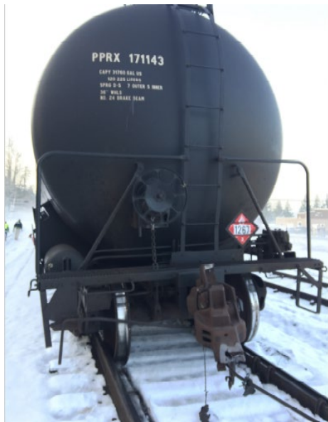
Broken coupler from car PPRX172350 attached to PPRX 171143.
