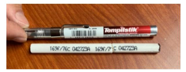
**Figure 1:** Exemplar Tempilstik issued to Train Crews. This will melt at hot wheel bearing temperatures of 169° or above. The inner wax-based, push-up crayon that will melt is removed and set below the pen in this photograph.
