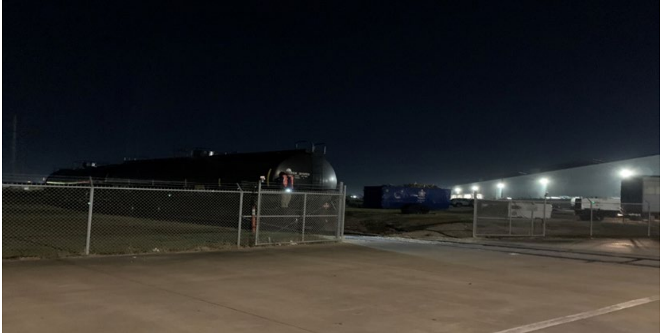
Figure 1: NTSB photograph taken during the site distance test conducted at 4:00 a.m. (the incident time) showing the incident Consist on the left, behind the open fencing gates. A NTSB investigator is standing on the Consist platform wearing an orange vest and white helmet and holding a lighted conductor's lantern. The white light on the rear of the Consist is a reflection of the building lights seen on the right side of the photograph.
