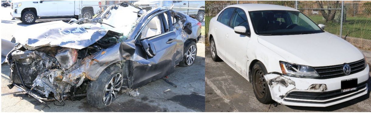
Figure 4. Postcrash damage to the 2017 Acura TLX (left) and the 2017 Volkswagen Jetta (right).
