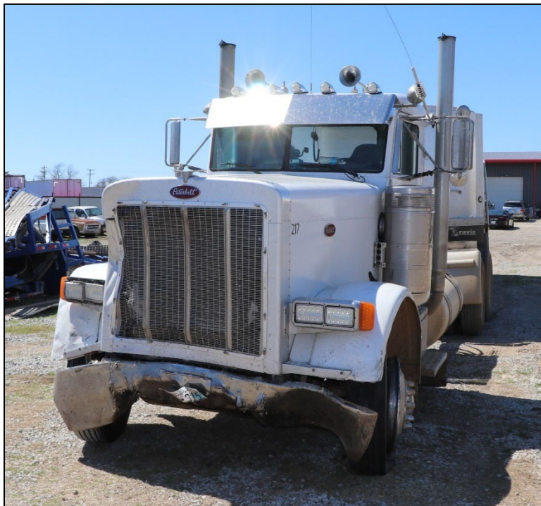
Figure 6. Postcrash photograph showing damage sustained by combination vehicle.
