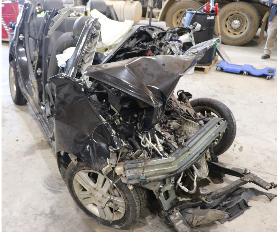
Figure 4. Postcrash photograph of damage to passenger car. The photograph was taken after the car had been moved to a garage. (Source: Oklahoma Department of Public Safety)
