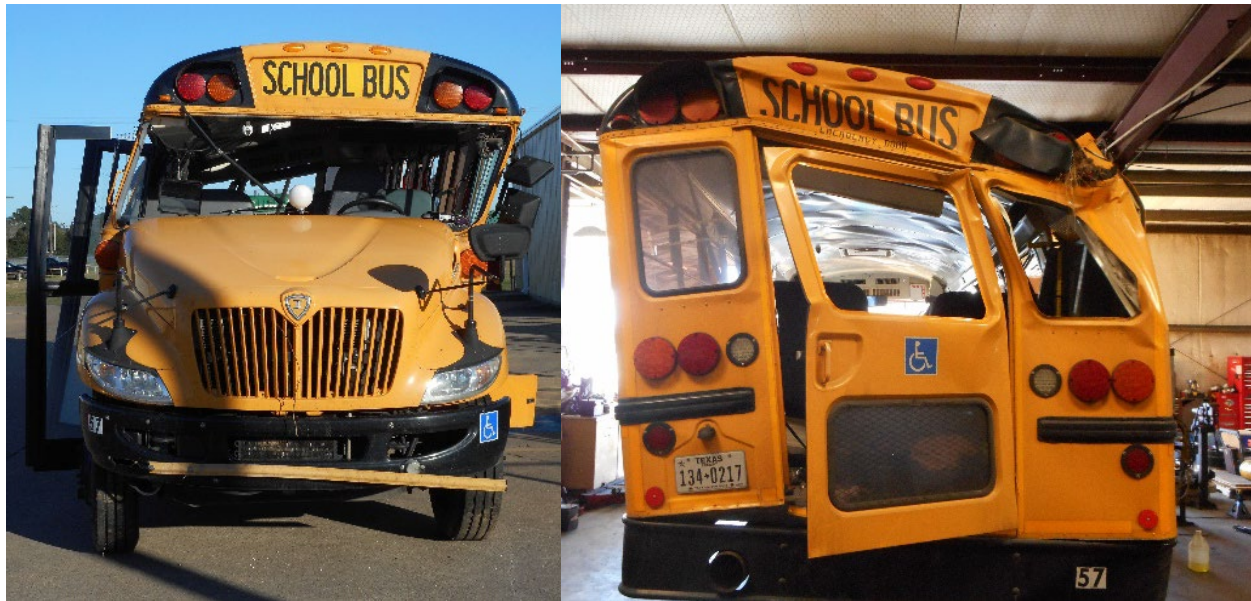
Figure 4. Front (left) and rear (right) view of school bus showing roof shift and damage to rear door.
