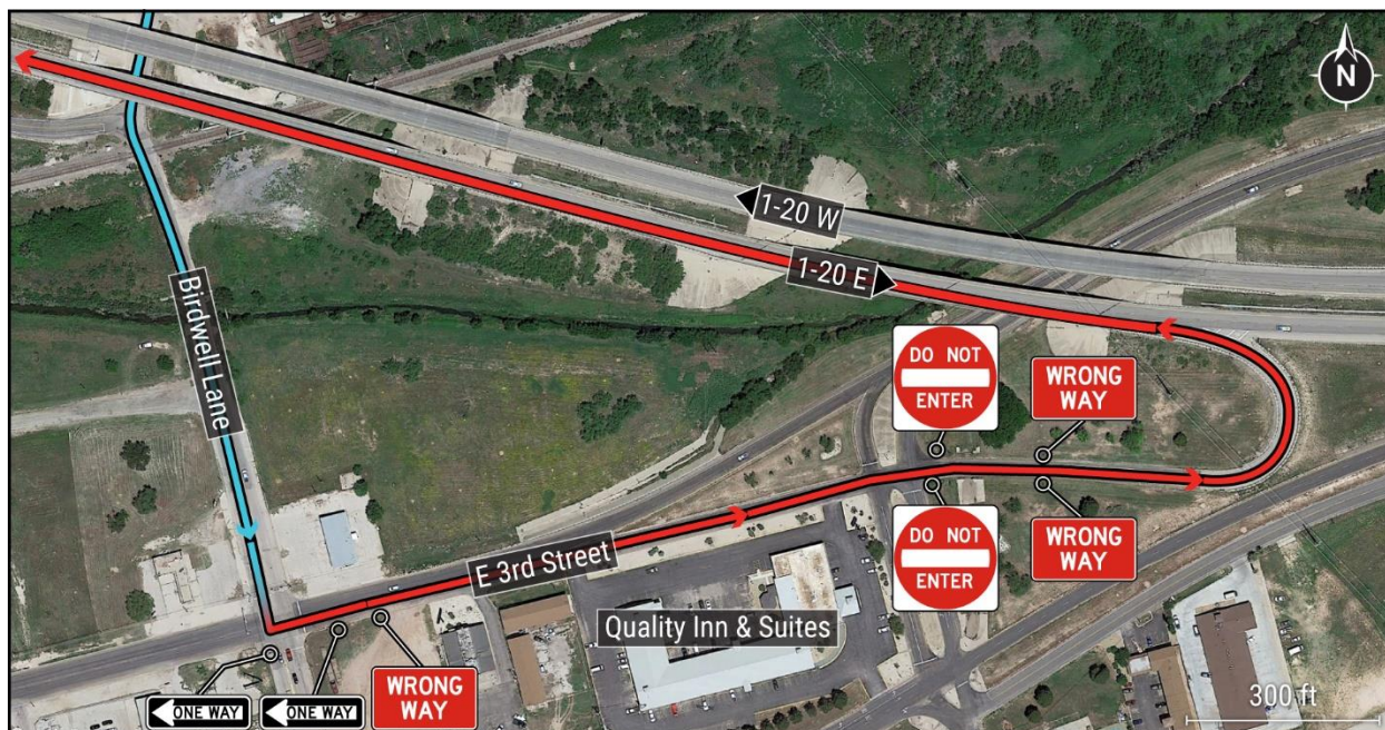
Figure 4. Traffic signs encountered by service truck driver indicating wrong-way travel from Birdwell Lane until he entered the exit ramp onto I-20. (Source: Google Maps; annotated by NTSB).
