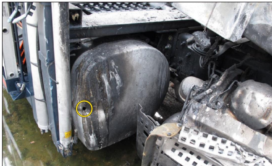
Figure 9. Fuel tank from passenger side of Volvo auto-transporter's truck-tractor, showing location of hole (circled in yellow) found in it postcrash.
